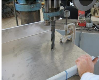
Figure 4.2. Drilling the hole on the sheet metal
