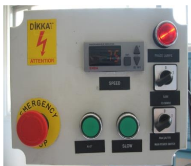
Figure 4.5. Control panel of the speed (rpm) adjusting device
