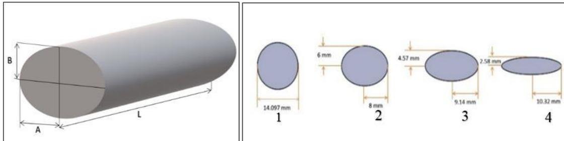
Figure (1): different tubes aspect ratio. Figure (2): Problem geometry and dimensions.
