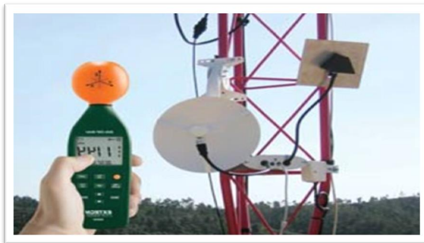
Fig.(4): RF EMF strength meter 480846
