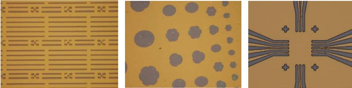
**Figure (2) : Results of the photolithography process**
