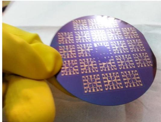
**Figure (3) : The Si/SiO<sub>2</sub> wafer after liftoff.**
