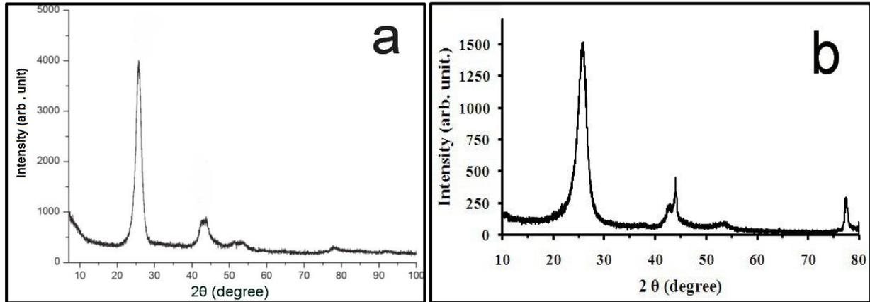
**Figure (6): XRD pattern of pure sample of a) SWCNTs, b) MWCNTs.**
