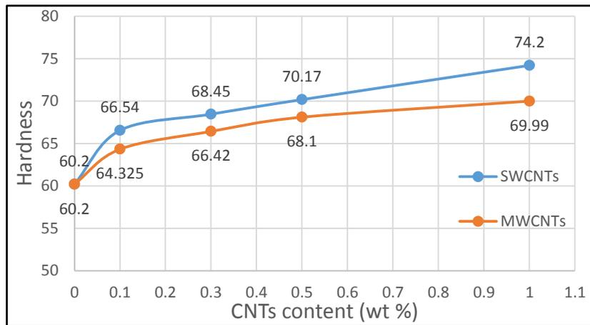
**Figure (11): Hardness of CNTs/Epoxy Composites.**
