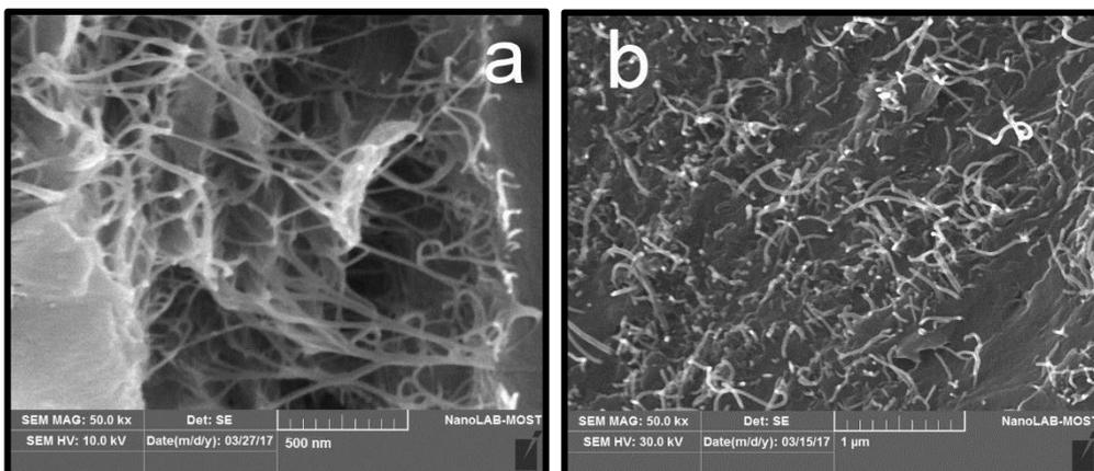
Finally, the images of SWCNTs/epoxy and MWCNTs/epoxy show the alignment of SWCNTs and MWCNTs into epoxy, this means that a good dispersion of each CNTs in this epoxy matrix and this agreement with the results Raman spectroscopy (Qing *et.al.*, 2008).
