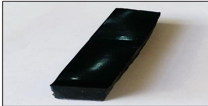
**Figure (1): CNTs/epoxy specimen.**
