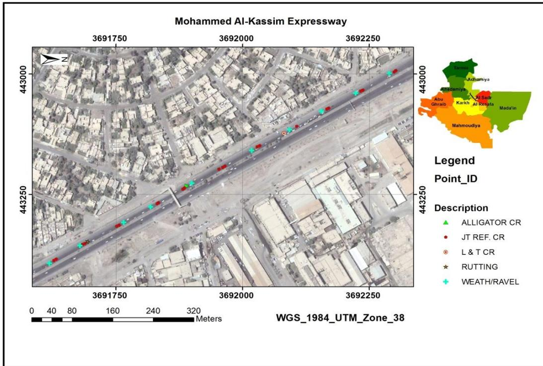
**Figure (13) Distress Types in AC Pavement Surface**
