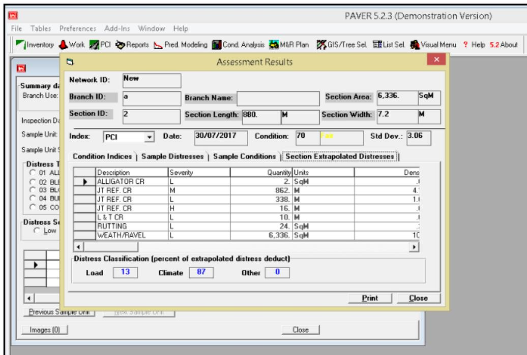
Figure (6) PCI of AC Pavement Surface with Distress Information and Classification
