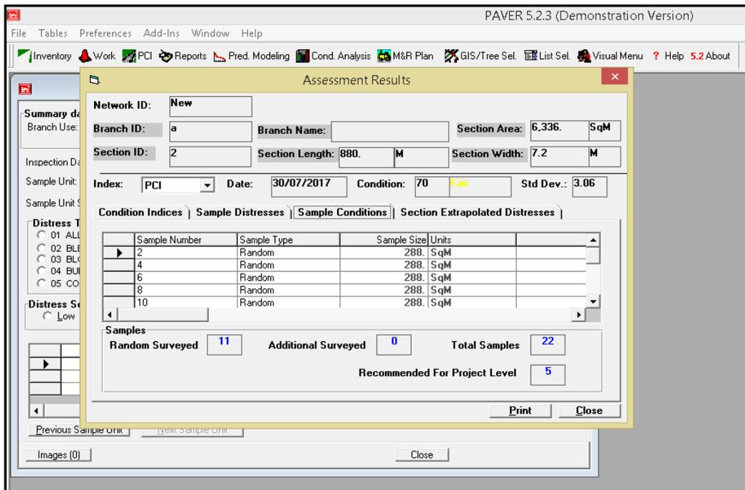
Figure (5) PCI for AC Pavement Surface and PCI for each Sample Unit with no. Sample Surveyed
