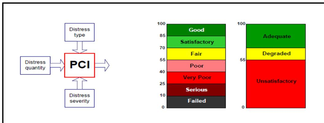
Figure (3) Pavement Condition Index (PCI) requirement, Ranges, and Suggested Colors [2]
