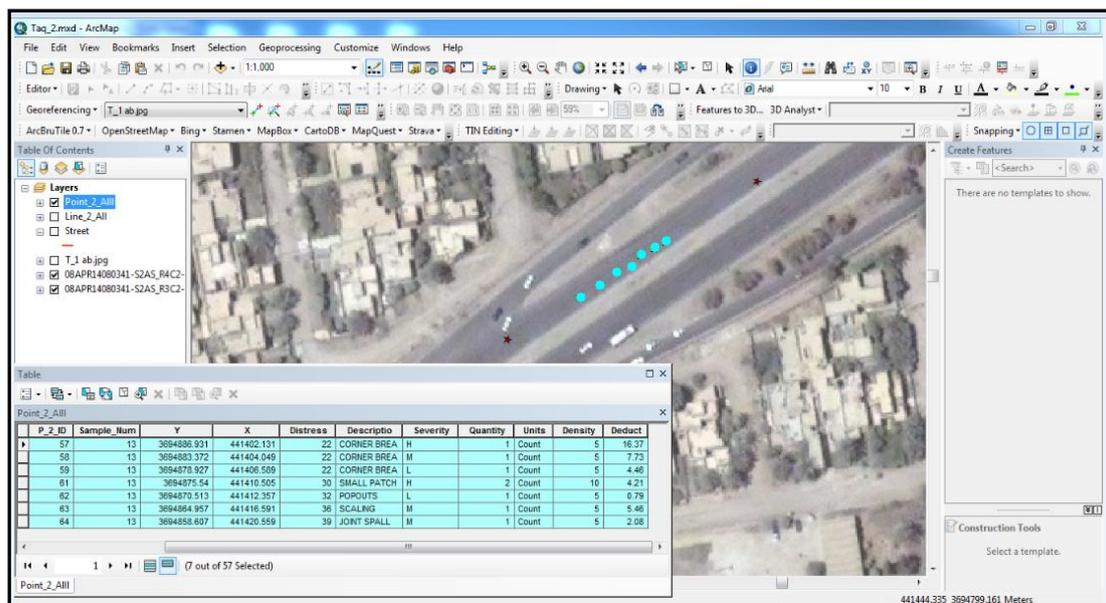
Figure (10) Database of distresses for sample unit 13 of Trans. Tining PCC Pavement Surface
