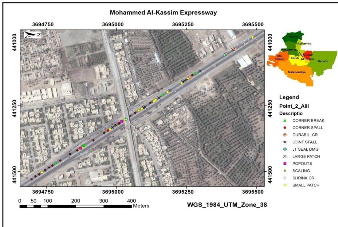
Figure (12) Distress Types in Transverse Tining PCC Pavement Surface
