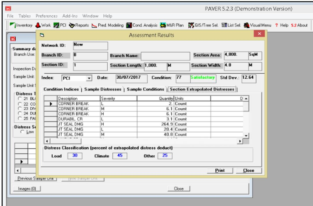
Figure (9) PCI for Transverse Tining PCC Pavement Surface with Distress Information and Classification
