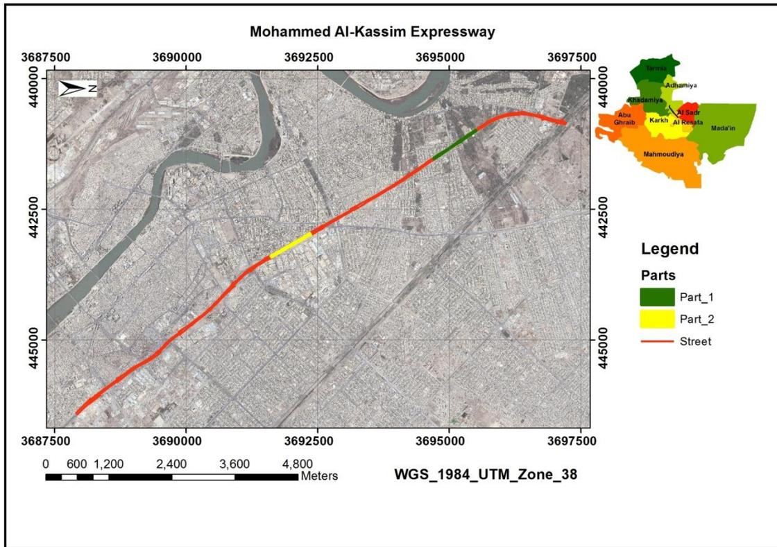
**Figure (1) Mohammed Al- Qassim Expressway (Part 1(Transverse Tining PCC pavement surface) Part 2 (AC pavement surface))**
