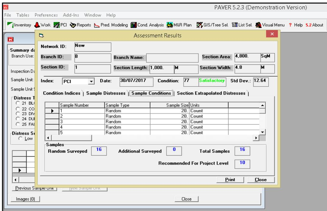
Figure (8) PCI for Transverse Tining PCC Pavement Surface and PCI for each Sample Unit with no. Sample Surveyed
