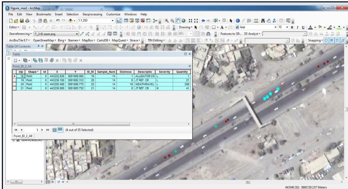
Figure (11) Database of distresses for sample unit 14 of AC Pavement Surface
