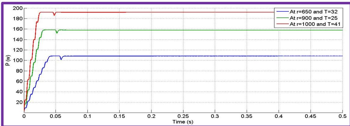
Figure 18 : Output Power of PV with P& O MPPT as Controller.
