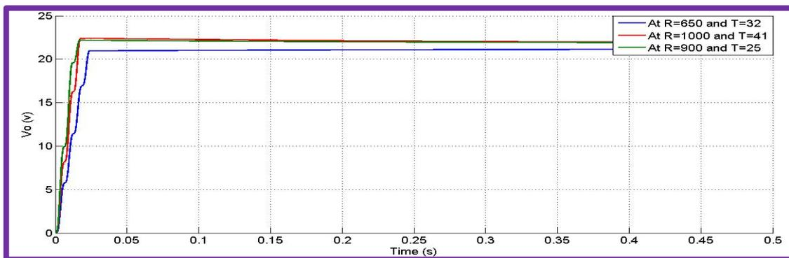
Figure 15 : Output Voltage of Buck Converter with PID Controller as MPPT.
