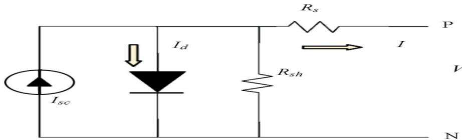
Figure 1 : PV mathematical model.(Joe-Air *et.al.*, 2005)
