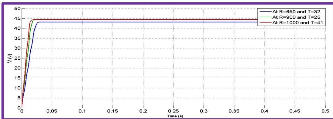
Figure 14 : Output Voltage of PV with P& O MPPT Controller.
