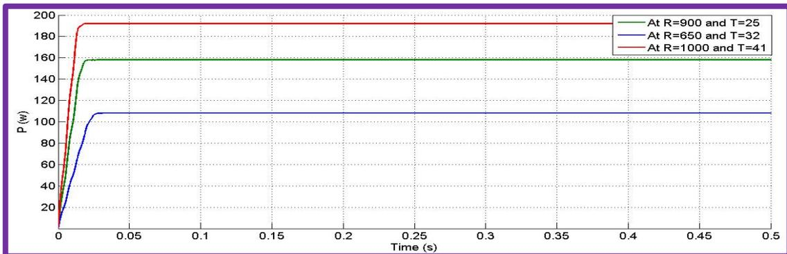
Figure 17 : Output Power of PV with PID Controller as MPPT.
