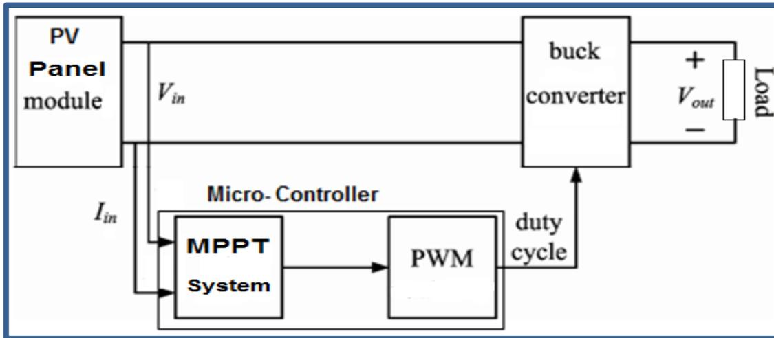
Figure 6 : Experimental System Model.
