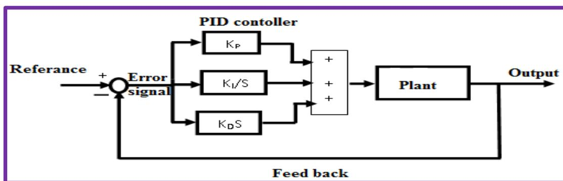
Figure 4 : Block Diagram of PID Controllers with plant.
