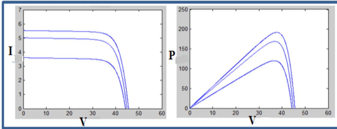
Figure 9 :V – I & V – P Relations of PV Panel.
