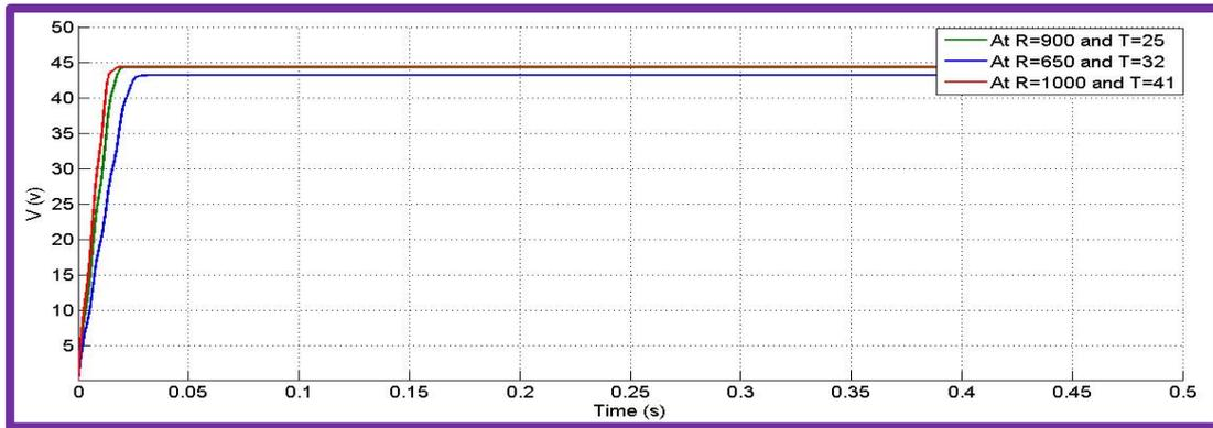
Figure 12 : Output Voltage of Buck Converter without MPPT.
