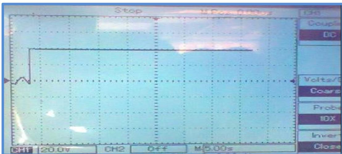
Figure 21: Output Voltage of PV Cell when  $T=41\text{ C}$  and  $R=995\text{w/m}^2$ .
