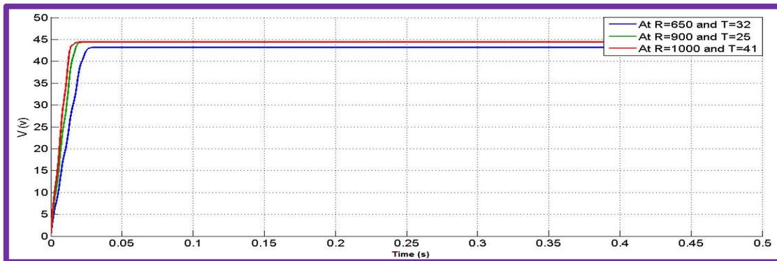
Figure 11: PV Voltage with Buck Converter.
