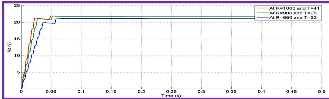
Figure 16 : Output Voltage of Buck Converter with P& O MPPT Controller.
