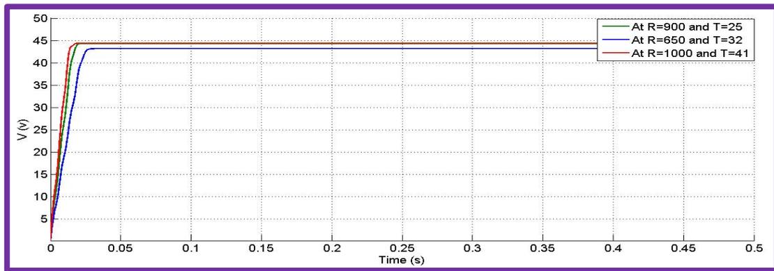
Figure 13 : Output Voltage of PV with PID Controller as MPPT.
