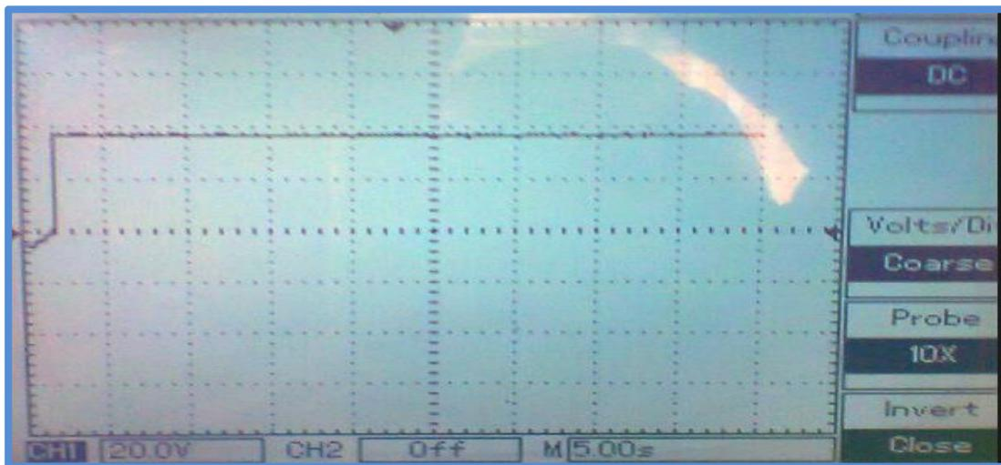
Figure 20 : Output Voltage of PV when  $T=25\text{ C}$  and  $R=900\text{w/m}^2$ .
