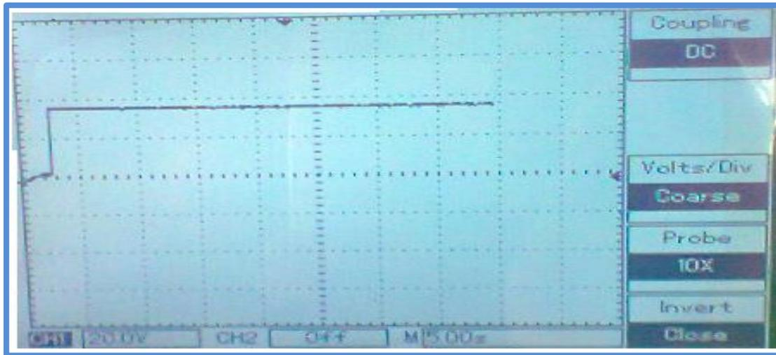
Figure 19 : Output Voltage of PV when  $T=32\text{ C}$  and  $R=650\text{w/m}^2$ .
