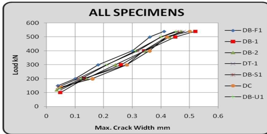
Figure (5) Crack Width For All Specimens
