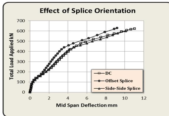
Figure (16) Load-Deflection Curves of Beams With Different Splice Orientations
