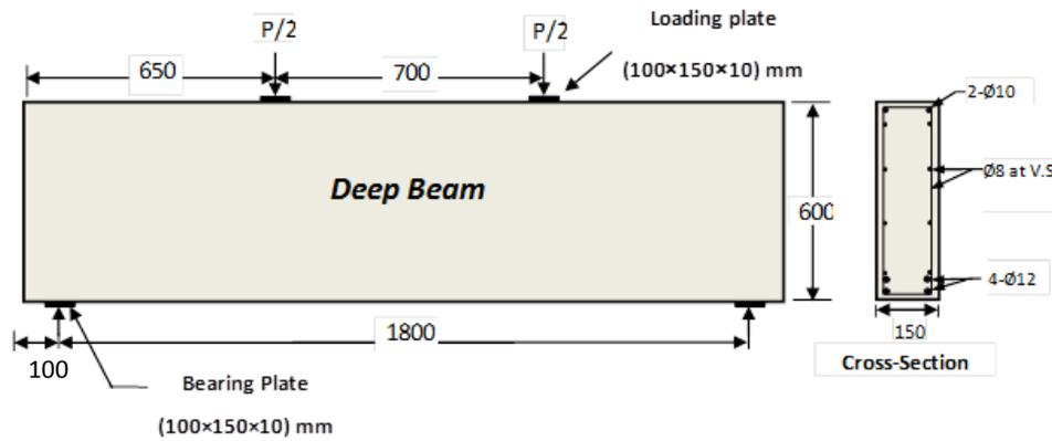
**Figure (1) Geometry and Loading Scheme of Tested Specimens**
