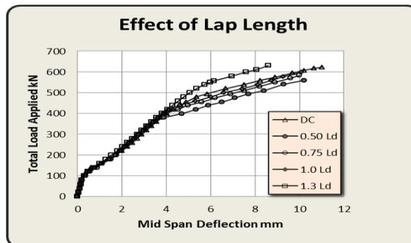
Figure (17) Load-Deflection Curves of Beams With Different Lap Length
