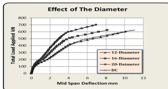
**Figure(14)Load-Deflection Curve of Beams With Different Diameter of Spliced Bar**
