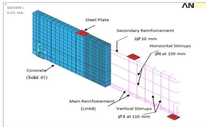
**Figure (9) Details Modeling of Beam Models**
