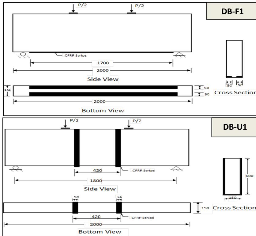
Figure (2) Details of Strengthened Beams With Lap Splices: DB-F1, DB-U1
