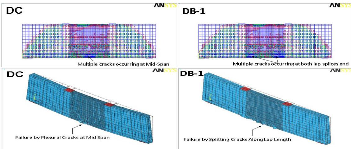
**Figure(12)Deformed Shape and Cracking Pattern at Ultimate Load For DB-1 &DC**
