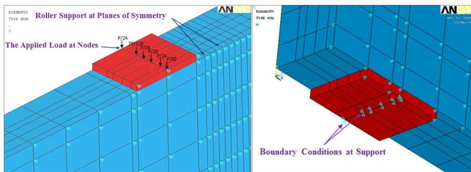
**Figure (10) Details of Boundary Conditions of (Symmetry, Supports and Loads)**
