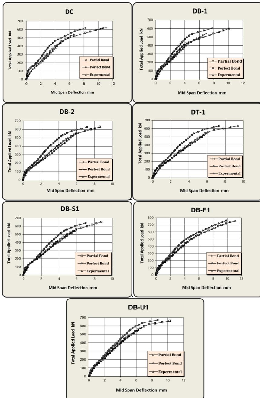
Figure (13) Load-Deflection Curve For All Specimens
