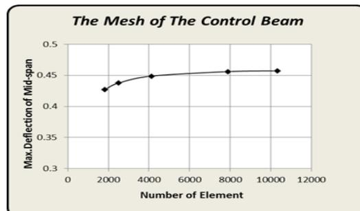
**Figure (8) Max. Deflection at Mid-Span Versus Number of Elements Relation Ship**
