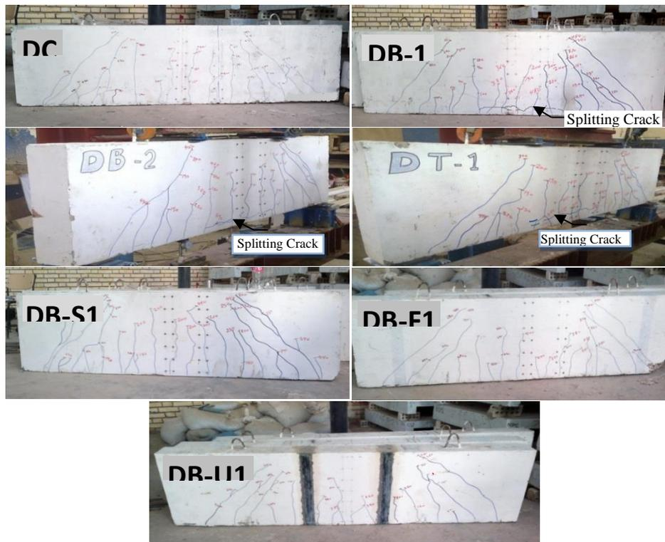
**Figure (4) Cracking Pattern For All Specimens.**
