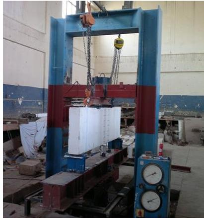
Figure (3) Testing Machine.
