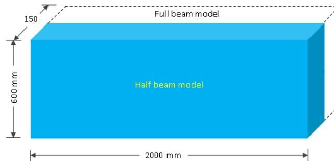
**Figure (7) Half Beam Finite Element Model**
