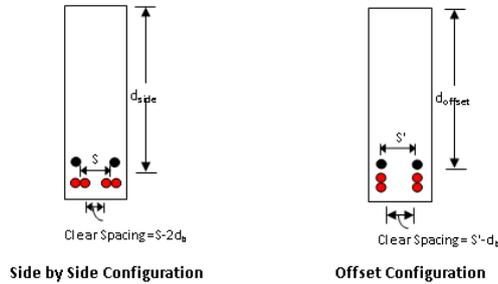
Figure (15) Clear Spacing Between Splices
