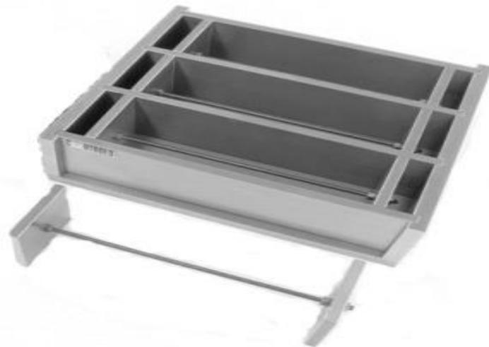
**Fig. 1. Mold with restraining cage**
