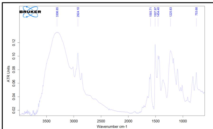
**Figure 5. FTIR test results of Novolac**
