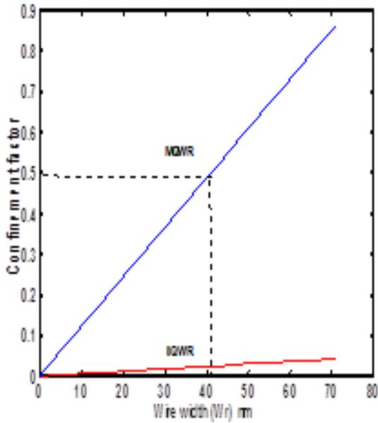
Fig.(4) The optical confinement factor as a function of the wire width for Al<sub>0.2</sub>Ga<sub>0.8</sub>As/ GaAs of MQWR structure.
