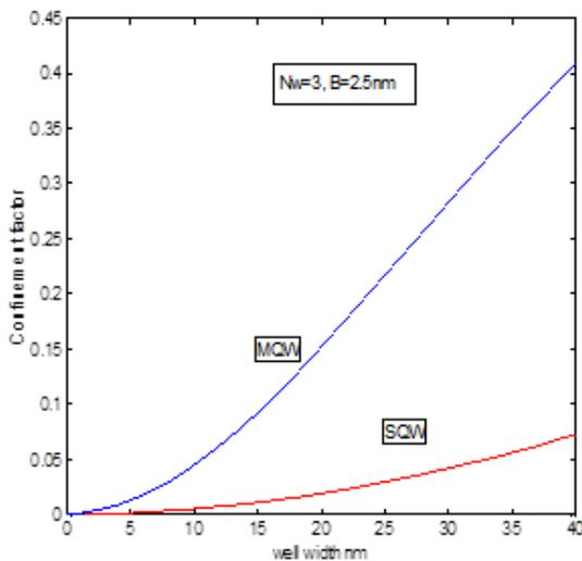
Fig.(3) The relation between confinement factor and well width of Al<sub>0.2</sub>Ga<sub>0.8</sub>As,  $x=0.2$ .
