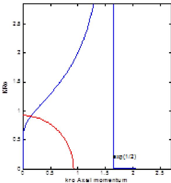
Fig.(5) The radius of the wire is reduced, the intersection moves toward the origin.
