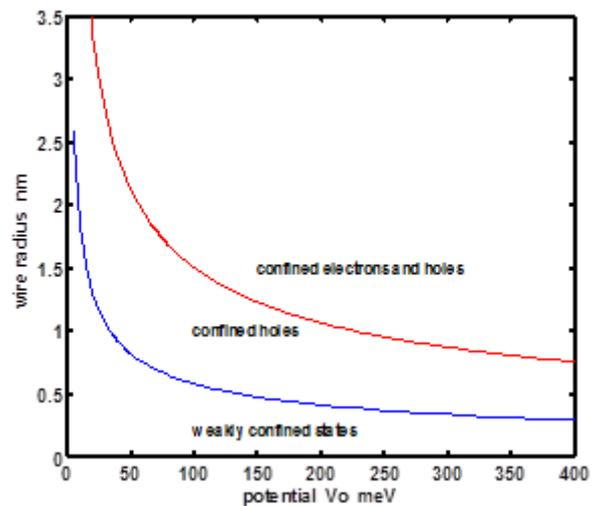
Fig.(8) Quasi-critical as a function of the band gap. Electrons and holes in quantum wires which are smaller than the quasi-critical radius are bound by the potential but are only weakly confined.
