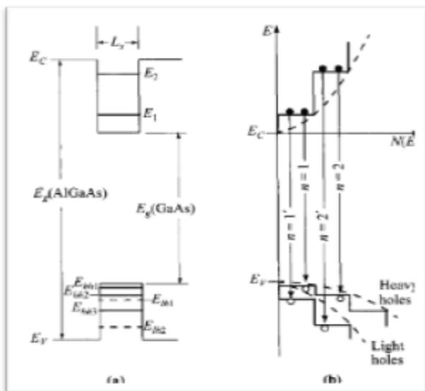
Fig.(2) (a) potential of quantum well and quantized levels.
