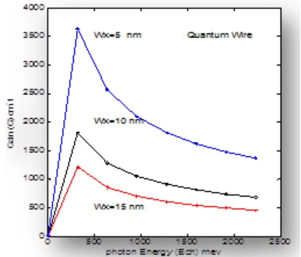
Fig.(7) The relation between the gain and photon Energy.
