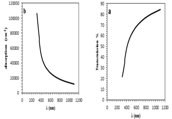
Fig (3) a) transmission of Bi<sub>2</sub>O<sub>3</sub> thin film b) absorption of Bi<sub>2</sub>O<sub>3</sub> thin film
