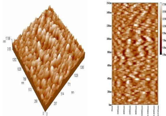
Fig (2) AFM image of Bi<sub>2</sub>O<sub>3</sub> thin film prepared at optimum condition
