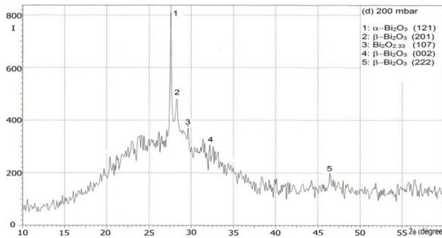
Fig (1) XRD of Bi<sub>2</sub>O<sub>3</sub> prepared by pulse laser deposition at specific preparation condition
