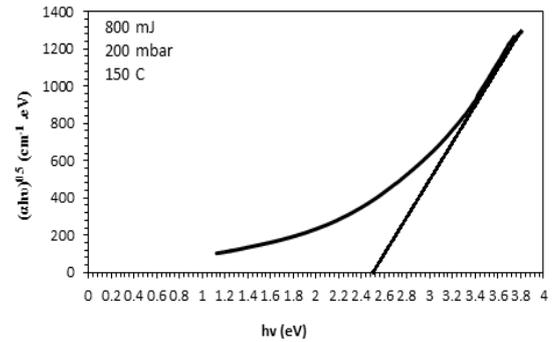
Fig (4) show the s a plot of  $(\alpha hv)^{1/2}$  versus  $h\nu$  for energy gap value for Bi<sub>2</sub>O<sub>3</sub> thin film
