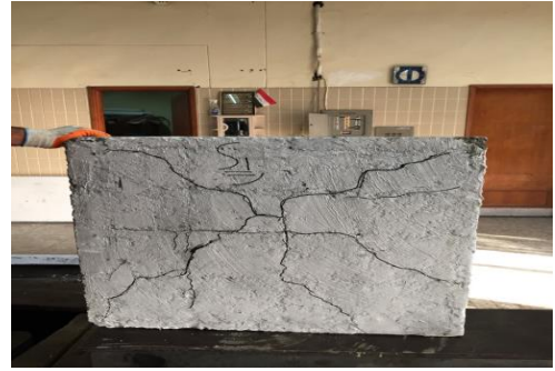
Figure 4.1: Slab (S1) after repairing and retesting
