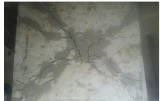
Figure 4.4 : Slab (S6) after repairing and retesting
