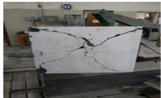
Figure 4.3 : Slab (S4) after repairing and retesting
