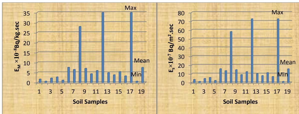
Fig. 4: (a) The mass exhalation rate ( $E_M$ ) of radon by unit Bq/kg.Sec, and b) The surface exhalation rate ( $E_S$ ) of radon by unit Bq/m<sup>2</sup>.sec. for all soil samples
