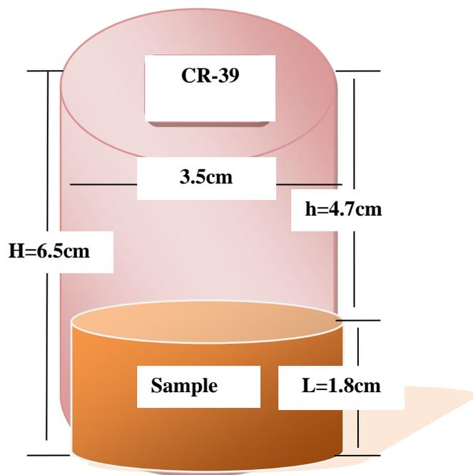
**Fig2: Test tube technique used in the study.**
