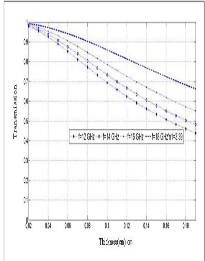
**Figure (13): Transmission as function to the thickness of slab for InGa Asp with different frequencies**
