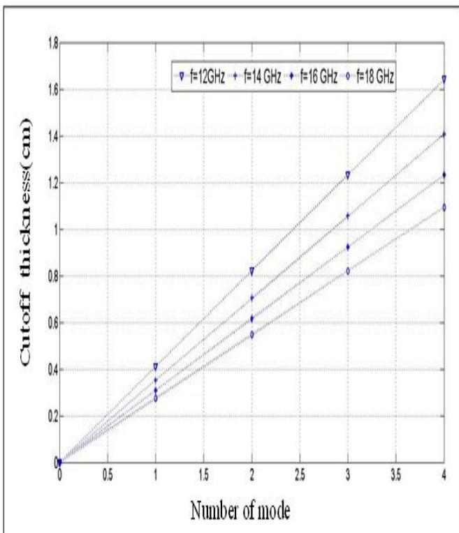
Figure (8) : Critical cutoff thickness as function to the number of modes for InGaAsP with  $n_2=1.5$ .
