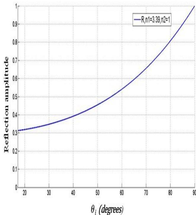
Figure (10): Reflection amplitude when incident angle( $\theta_i$ ) is greater than critical angle for InGaAsP and  $n_2=1$ .
