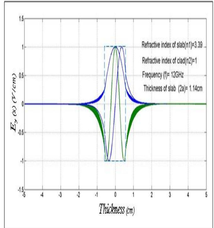
**Figure (5): TE( $m=0,1,2$ ) mode in InGaAsP waveguide with thickness 1.14 cm at 12 GHz  $n_1=3.39$  for ,  $n_2=1$  .**
