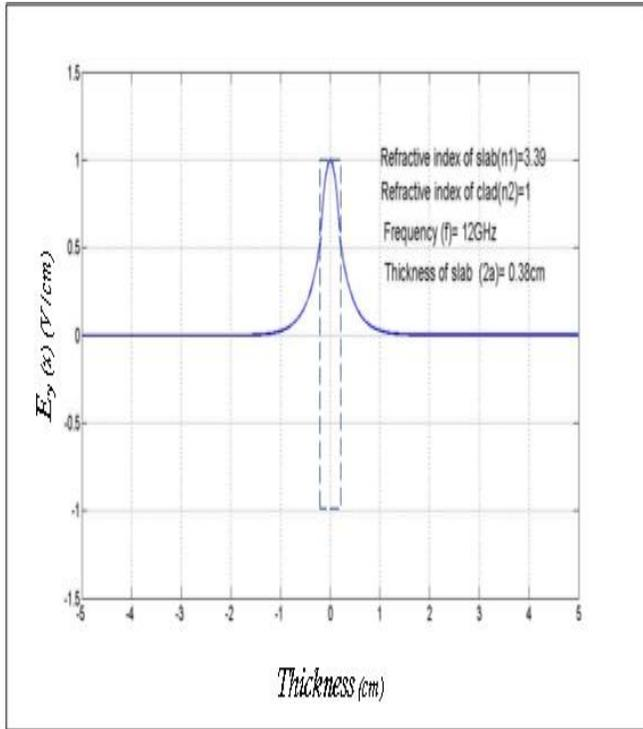
**Figure (3): TE( $m=0$ ) mode in InGaAsP waveguide with thickness 0.38cm at 12 GHz for  $n_1=3.39$ ,  $n_2=1$ .**
