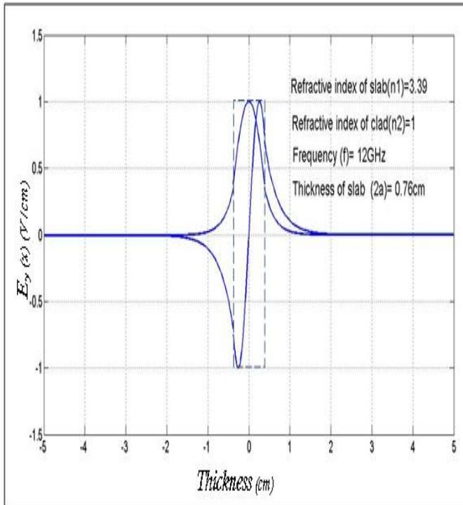
**Figure (4): TE( $m=0,1$ ) mode InGaAsP waveguide with thickness 0.76 cm at 12 GHz for  $n_1=3.39$ ,  $n_2=1$ .**
