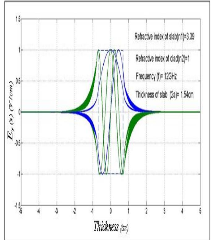
**Figure (6): TE( $m=0,1,2,3$ ) mode in InGaAsP waveguide with thickness 1.54 cm at 12 GHz for  $n_1=3.39$ ,  $n_2=1$  .**
