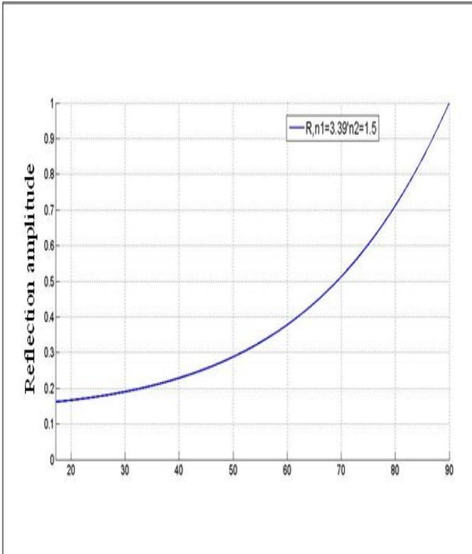
**Figure (11): Reflection amplitude when incident angle( $\theta_i$ ) is greater than critical angle for InGaAsP and  $n_2=1.5$ .**
