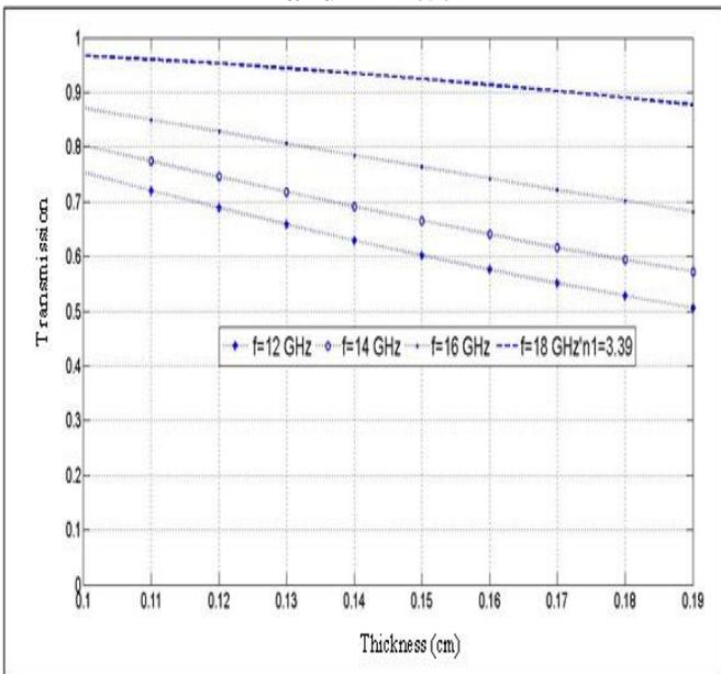
**Figure (12): Transmission as function to the thickness of the slab for InGaAsP sample with different frequencies.**
