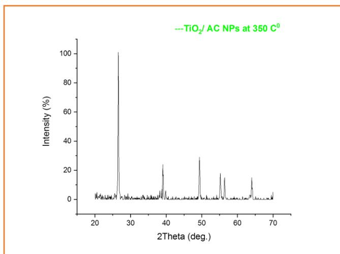
**Figure (3): TiO<sub>2</sub>/AC nanocomposites XRD spectra.**
