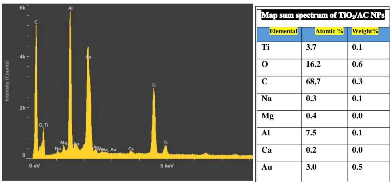
**Figure (5): Pure TiO<sub>2</sub>/AC NPs elemental mapping and EDX analysis.**
