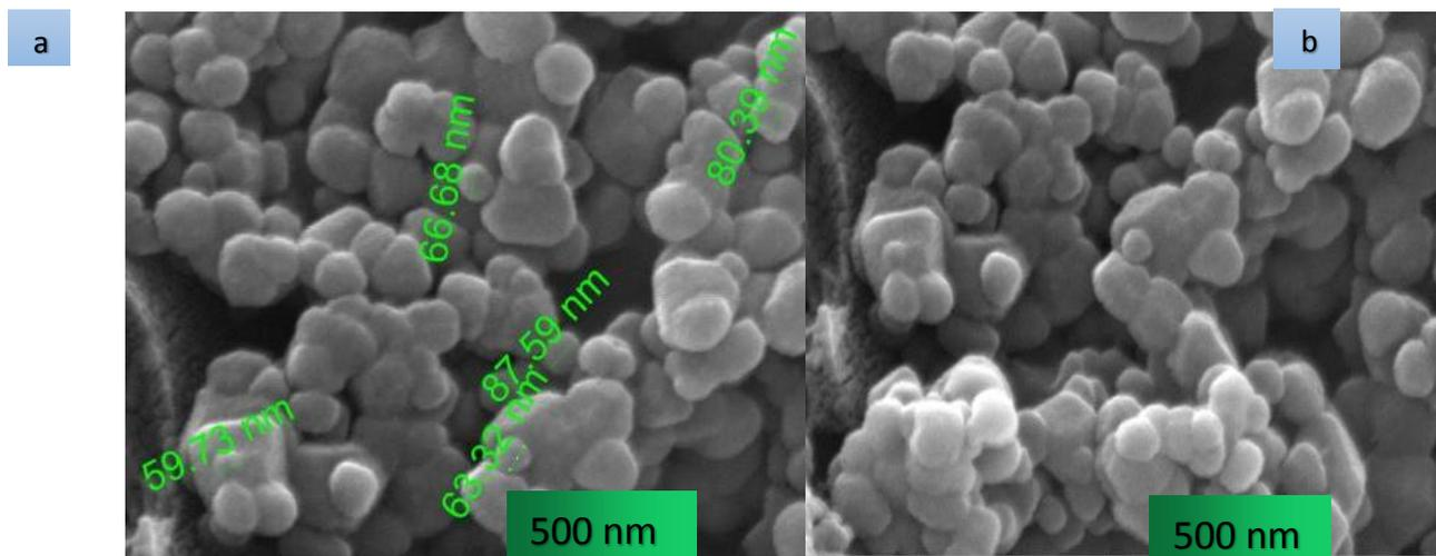
**Figure.4:** (a) and (b) TiO<sub>2</sub>/AC nanocomposite image captured by FE-SEM with particle size and without respectively .
