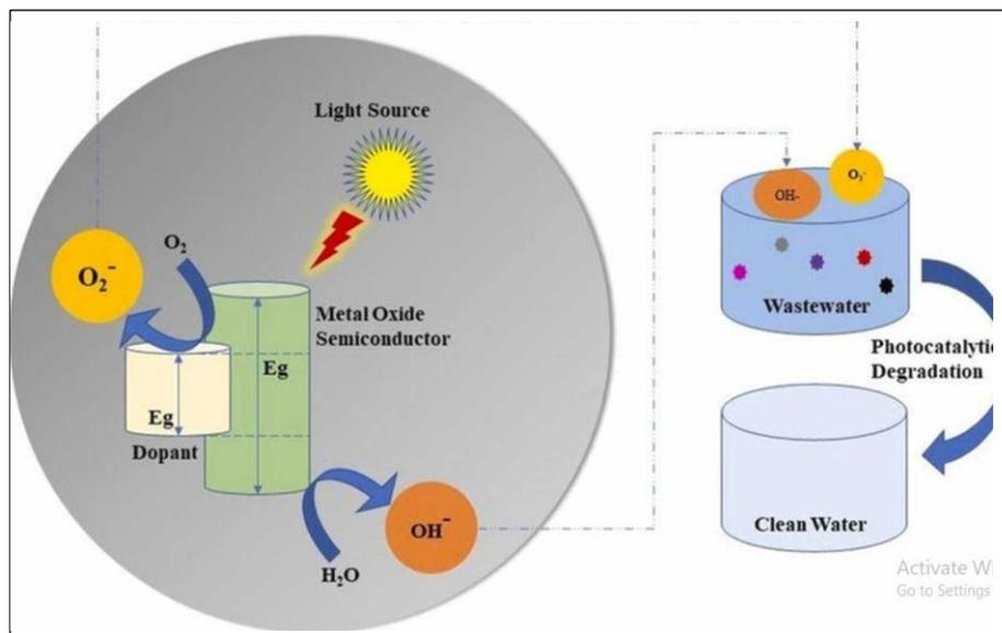
**Figure (1): Diagram schematic for photocatalyst photoactivation[8].**
