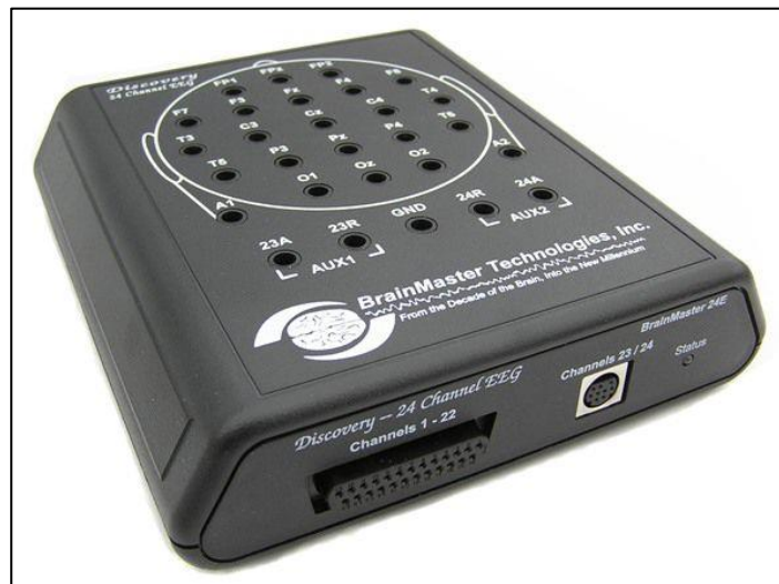
Figure 1: Brain Master Discovery 20 with Impedance Lid BrainAvatar 4.0 Discovery Acquisition system.
