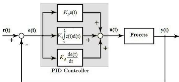
Fig (1) PID Controlled System
