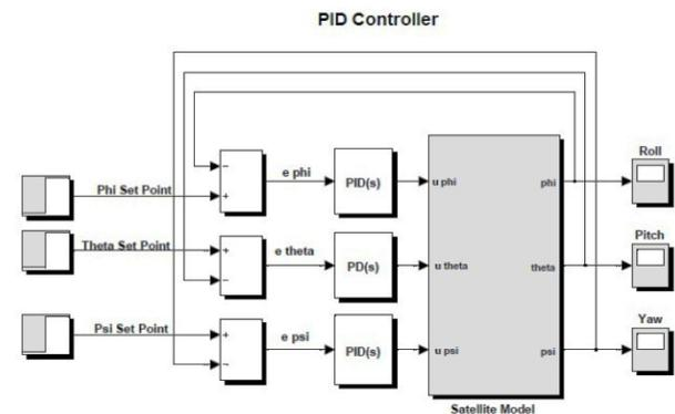
Fig (2) SIMULINK diagram of satellite model with PID controller
