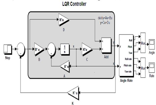
Fig (3) SIMULINK diagram of satellite model with LQR controller
