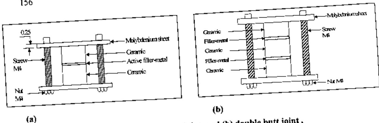
Fig. 1 Fixtures for (a) single butt joint and (b) double butt joint .
