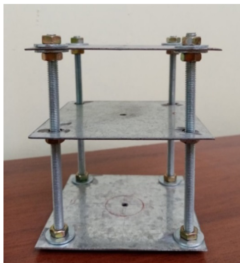
Figure (1) hand-made tool use to expose the detector with different energy by changing the distances between the source and the detector.
