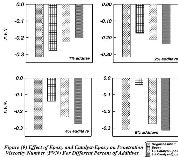
Figure (9) Effect of Epoxy and Catalyst-Epoxy on Penetration Viscosity Number (PVN) For Different Percent of Additives
