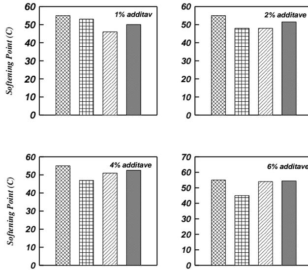
Figure (5) Effect of Epoxy and Catalyst-Epoxy on Softening Point For Different Percent of Additives
