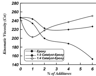
Figure(6) Effect of Epoxy and Catalyst-Epoxy on Kinematic Viscosity @ 135C
