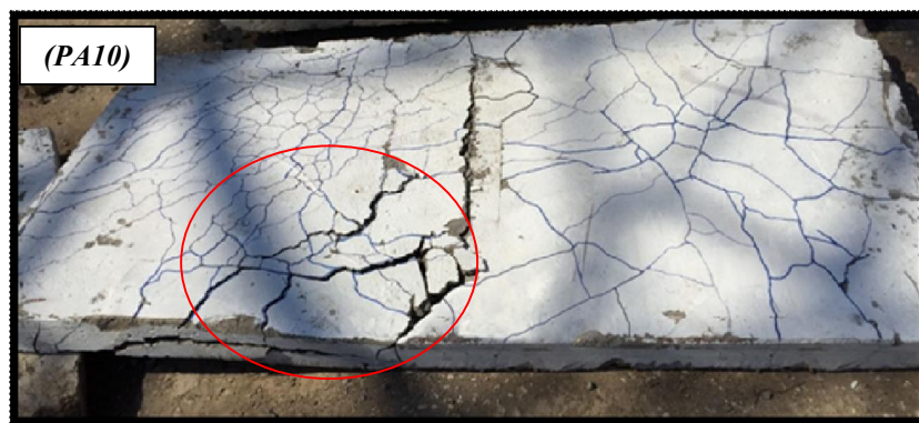
Figure (12): Crack pattern ( D/t = 0.6 ) (PA10).
