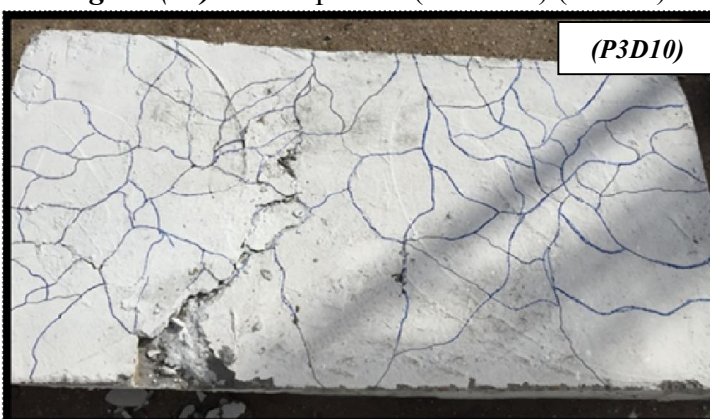
Figure (16): Crack pattern ( D/t = 0.6 ) (P3D10).
