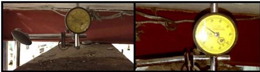
Figure (5): Dial Gauge Used to Measuring Deflection.
