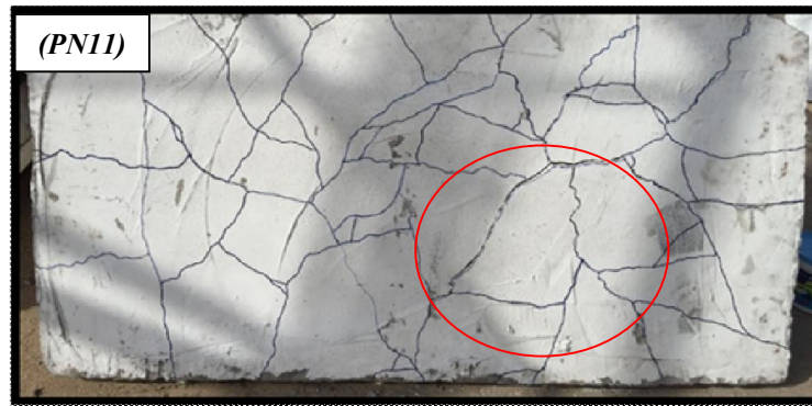
Figure (19): Crack pattern ( D/t = 0.7 ) (PN11).
