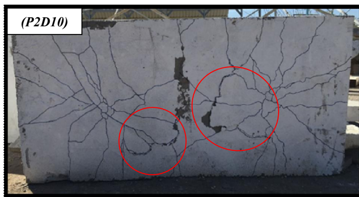
Figure (14): Crack pattern ( D/t = 0.6 ) (P2D10).
