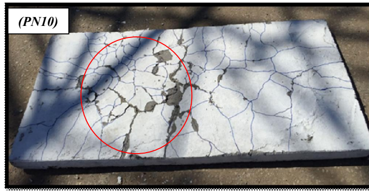
Figure (18): Crack pattern ( D/t = 0.6 ) (PN10).
