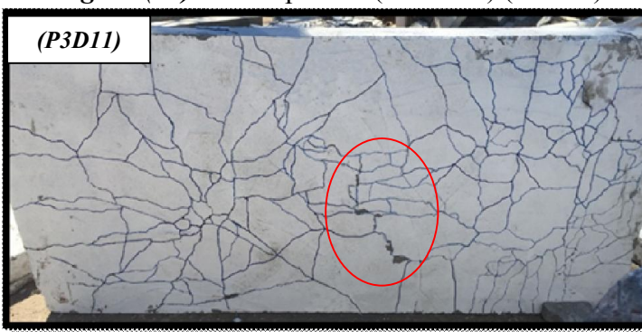
Figure (17): Crack pattern ( D/t = 0.7 ) (P3D11).
