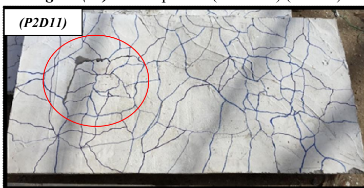
Figure (15): Crack pattern ( D/t = 0.7 ) (P2D11).
