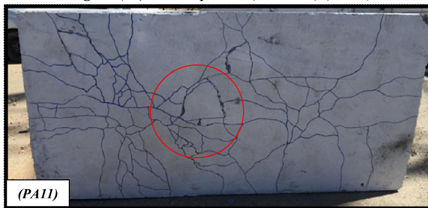
Figure (13): Crack pattern ( D/t = 0.7 ) (PA11).
