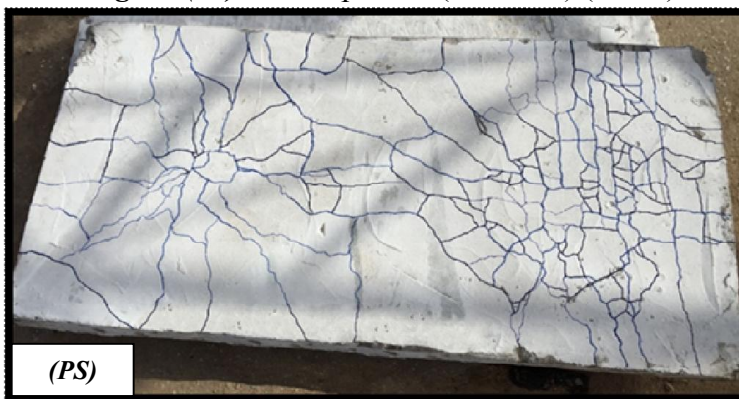
Figure (20): Crack pattern at the ultimate load for continuous RPC solid slab and 10 cm slab thickness (PS).
