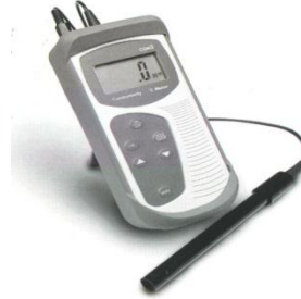
(b) Portable pH/°C Meter (OAKTON, 1999)
