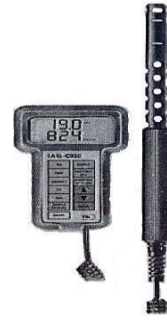
(a) Indoor Air Quality Meter IAQ-CALC (TSI, 2004)
