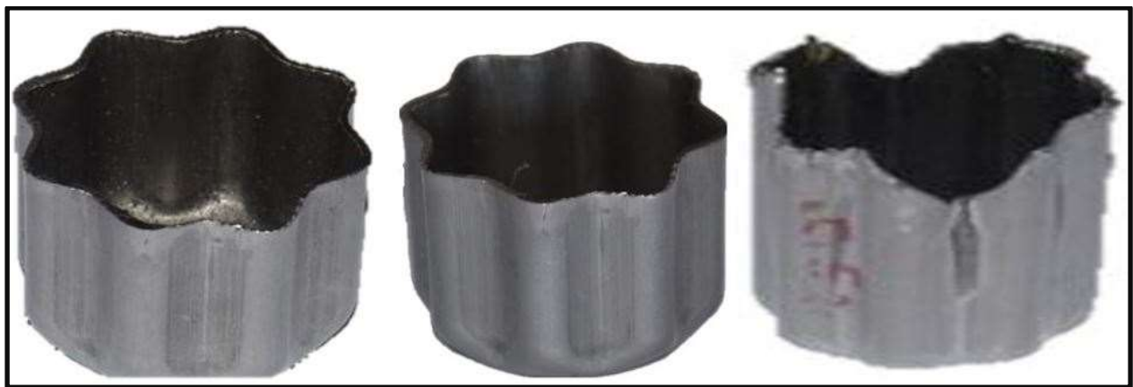
Figure 8: The astral cup produced with different radial clearance
