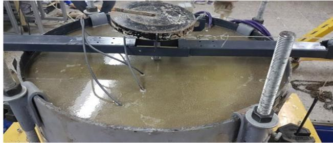
Plate 4: liquefaction phenomena occurred after applying 0.32g acceleration
