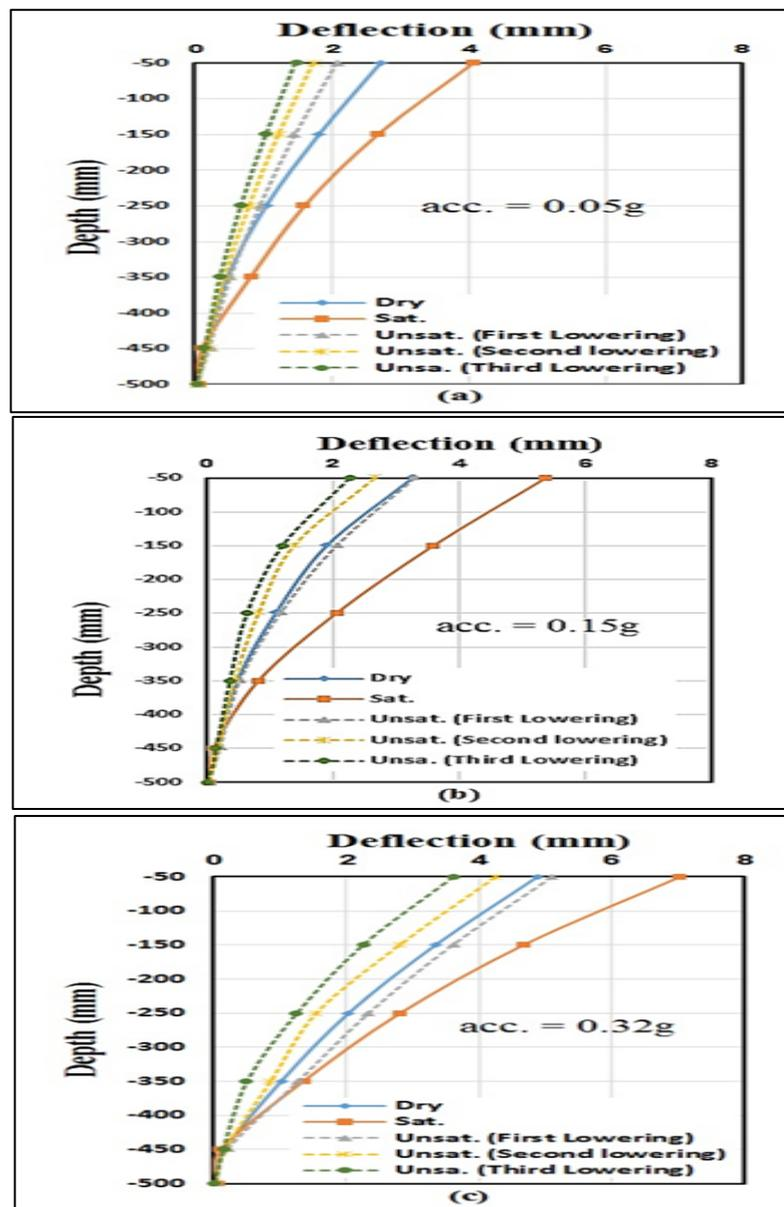
Figure 6: Deflection of single pile model under acceleration of lateral shaking 0.15g, (c) 0.32g and load (earthquake) of (a) 0.05g, (b) embedded in cohesionless soil of different saturation condition
