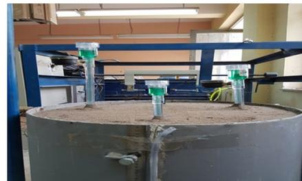
Plate 2: Soil suction test by LT Tensiometer
