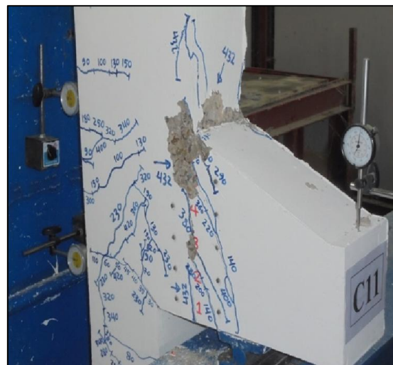
Fig.7 (b) Failure Mode of Specimen C11
