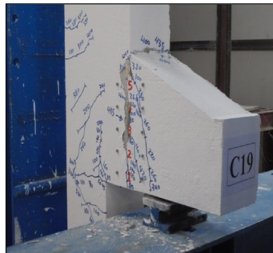
Fig.11 (b) Failure Mode of Specimen C19
