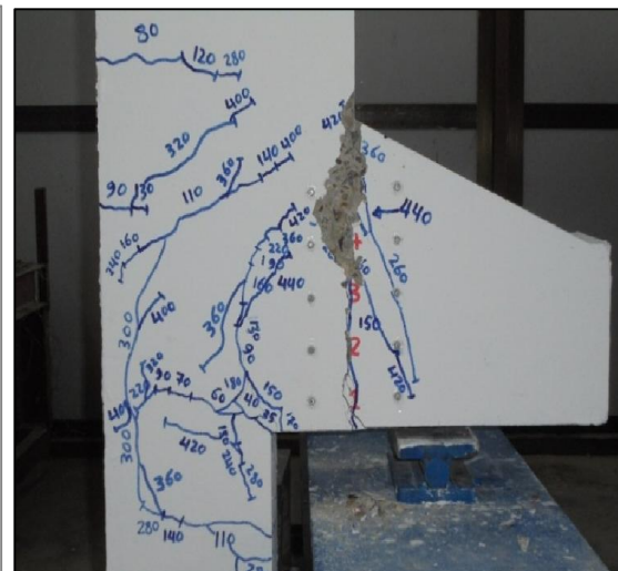
Fig.8 (b) Failure Mode of Specimen C12
