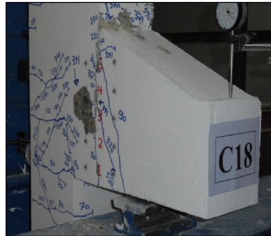
Fig. 10 (b) Failure Mode of Specimen C18
