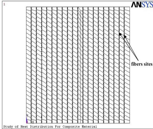
Fig (2-a) finite element mesh, fibers angled at  $0^\circ$  with the load direction
