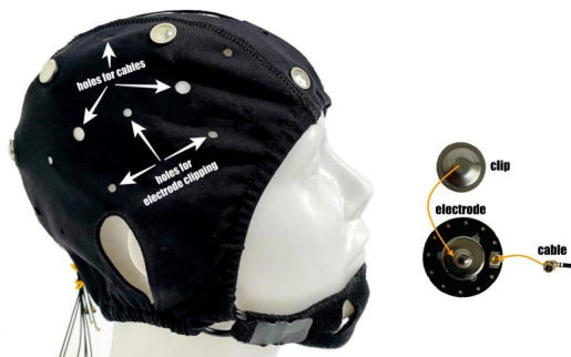
Figure 3: BrainAccess cap with dry-contact EEG electrodes.
