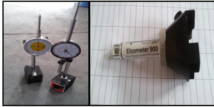
(b) Mechanical Extensometer (c) Micro Cracks Reader
