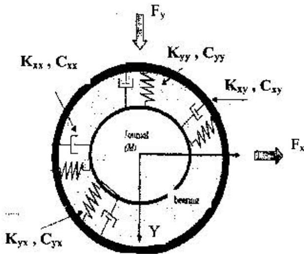
**Fig.2 Representation of point mass and bearing force coefficients**
