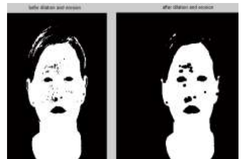
Figure (4): The effect of dilation and erosion on an image of system data base.
