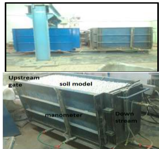
Plate 2: Two soil model containers were manufactured for soaking and leaching processes.
