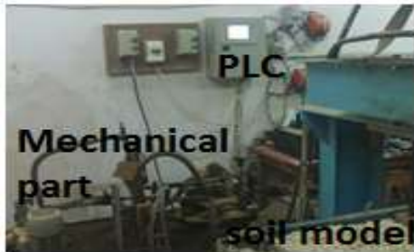
Plate 3 Computerized PLC of monotonic and repeated apparatus system with physical soil model during testing.
