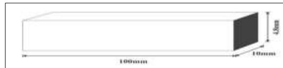
Dimensions samples of the flexural test
