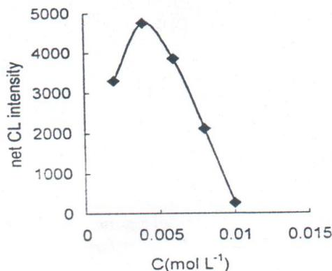
Fig. 5. The effect of  $K_3Fe(CN)_6$  concentration
