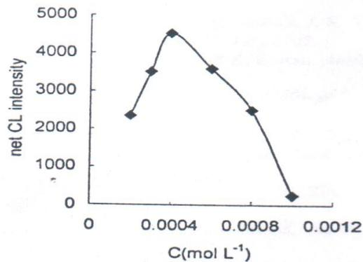
Fig. 3. The effect of luminol concentration
