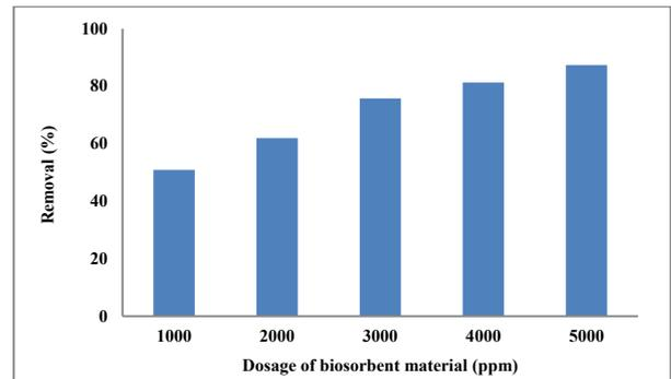
Figure 4: Effect of adsorbent dosage on removal percentage of crude oil at different adsorbent dosage, pH 6.18, 250 rpm, 25 °C, initial crude oil concentration 257.06 ppm and contact time 90 minutes
