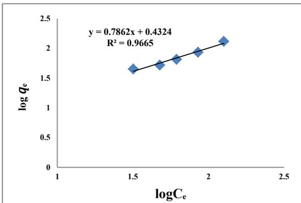
Figure 6: Linearized Freundlich isotherm model plot for biosorption of crude oil at pH 6.18, initial crude oil concentration 257.06 ppm, 250 rpm and 25 °C.
