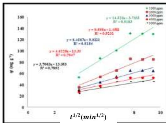
Figure 10: Intraparticle diffusion model plot for different adsorbent dosage addition on biosorption of crude oil at pH 6.18, initial crude oil concentration 257.06 ppm, 250 rpm and 25 °C
