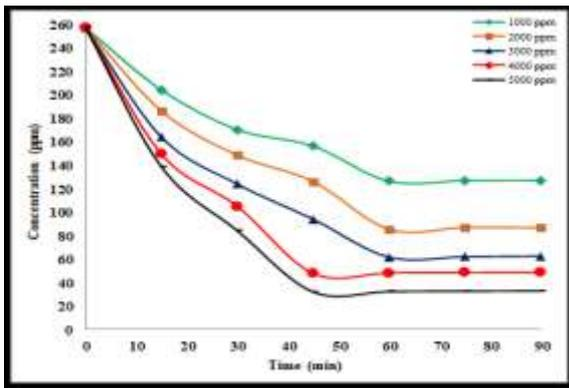
Figure 3a: Effect of contact time on the concentration of crude oil at different adsorbent dosage concentration, pH 6.18, 250 rpm, 25 °C and initial crude oil concentration 257.06 ppm
