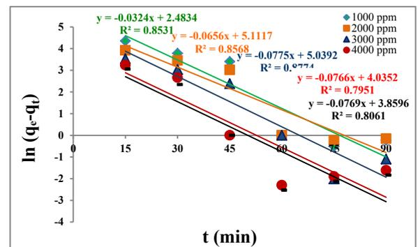
Figure 8: Pseudo-first-order kinetic model plot for different adsorbent dosage addition on biosorption of crude oil at pH 6.18, initial crude oil concentration 257.06 ppm, 250 rpm and 25 °C.
