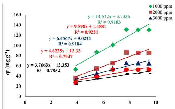
Figure 9: Pseudo-second-order kinetic model plot for different adsorbent dosage addition on biosorption of crude oil at pH 6.18, initial crude oil concentration 257.06 ppm, 250 rpm and 25 °C.
