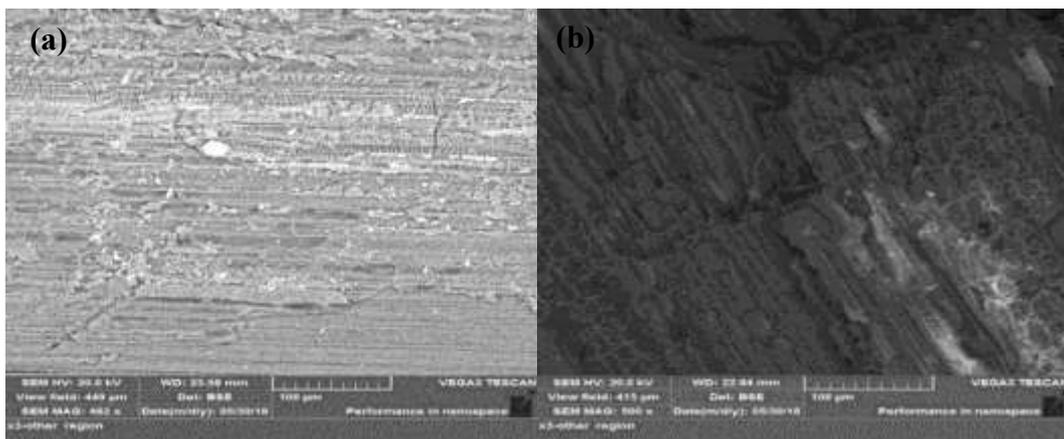
Figure 2: Scanning Electron Microscopy (SEM) analysis of papyrus reeds (a) before and (b) after crude oil adsorption
