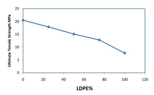
Fig.(2):Ultimate tensile strength of PP/ LDPE blend.
