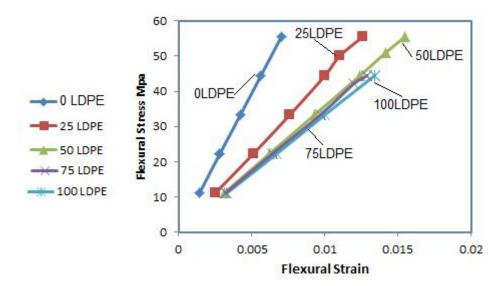
Fig.(4): Flexural stress and flexural strain for PP/LDPE.
