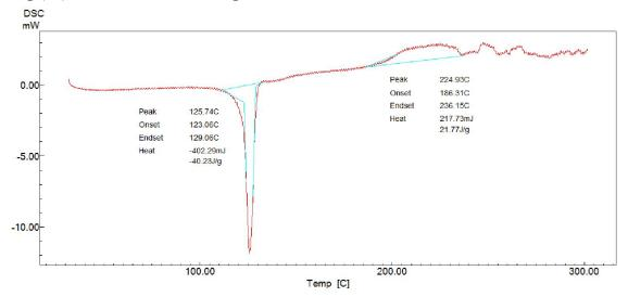
Fig.(12):-Differential scanning calorimeter curve for pure LDPE.
