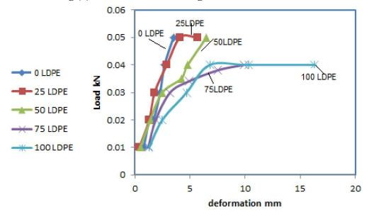
Fig.(3):Load -deformation for three points flexural test of PP/LDPE blend.
