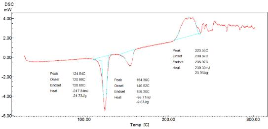
Fig.(10):-Differential scanning calorimeter curve for 50 LDPE / 50 PP.
