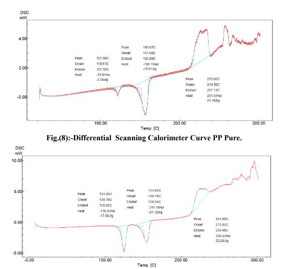
Fig.(9):-Differential Scanning Calorimeter curve for 25 LDPE /75 PP.
