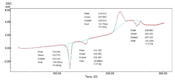
Fig.(11):-Differential scanning calorimeter curve for 75 LDPE / 25 PP.
