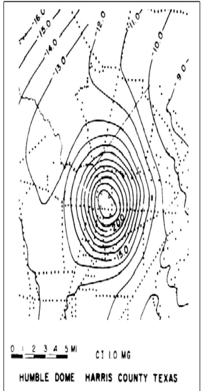
Fig. (13) Bouguer gravity map, Humble salt dome, Harris County, Texas, USA, after (12).
