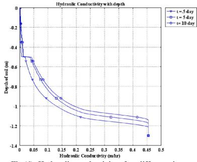
Fig.(6): Hydraulic conductivity after different time.
