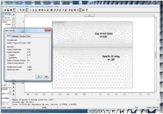
Fig.(2): Domain discrezation of unconfined aquifer.
