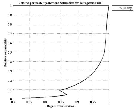
Fig.(8): Relative permeability-Benzene saturation curve of heterogeneous soil. 8. Conclusions
