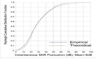
Figure 4: SNR fluctuation per RB in a Rayleigh distributed channel
