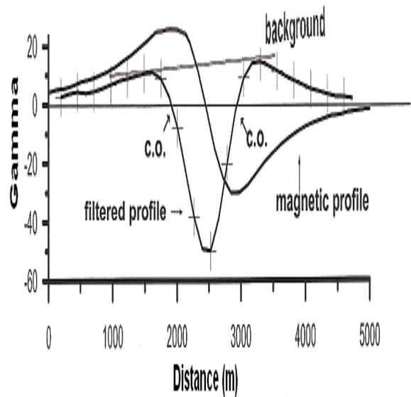
**Fig.(3a) Magnetic anomaly profile for dyke-like body (depth 500, width 500, inclination angle 40°) with its filtered profile using Fraser filter.**
