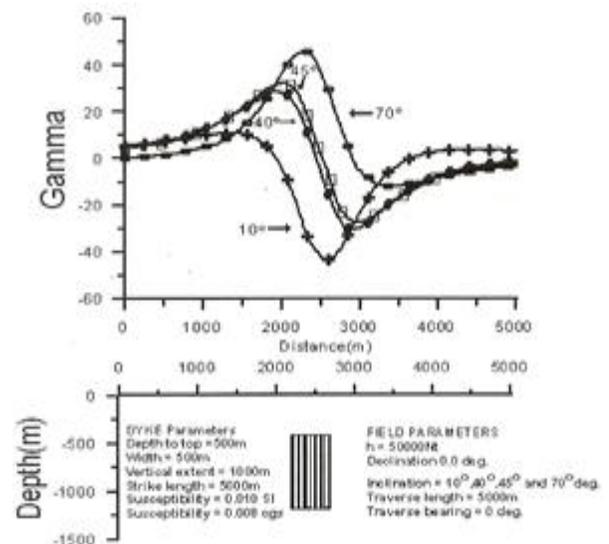
**Fig.(1) Total magnetic anomaly profile for dyke-like body with inclination angles 10,40,45,and 70 degrees.**
