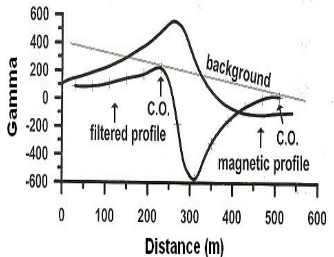
**Fig.(8a)** Field example of the total magnetic profile and its filtered profile obtained by applying Fraser filter. ( magnetic anomaly after Kara et.al. 2003)
