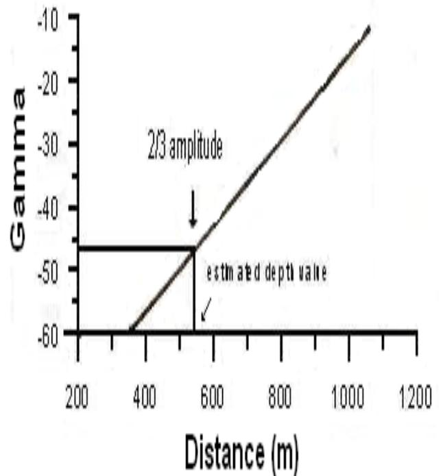
Fig.(5c) Depth estimation of dyke-like body from the relation of various amplitudes against distances between two straight lines of filtered profile.
