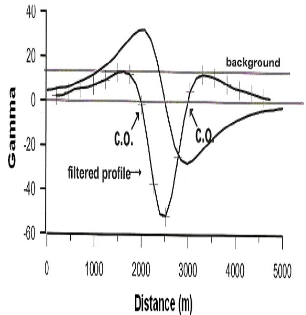
Fig.(4a) Magnetic anomaly profile for dyke-like body (depth 500, width 500, inclination angle 45o) with its filtered profile using Fraser filter.
