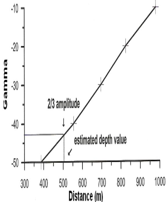
Fig.(3c) Depth estimation of dyke-like body from the relation of various amplitudes against distances between two straight lines of filtered profile.
