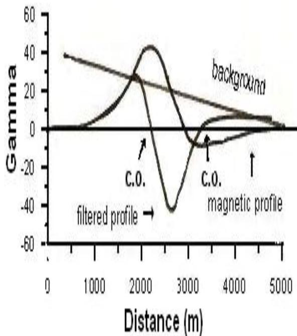
Fig.(5a) Magnetic anomaly profile for dyke-like body (depth 500, width 500, inclination angle 70o) with its filtered profile using Fraser filter.
