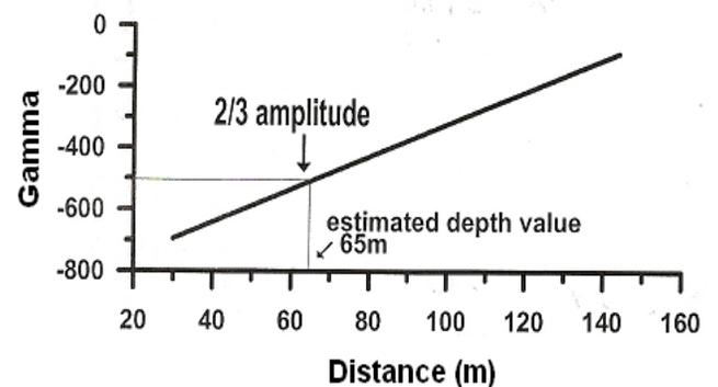
**Fig.(8c)** Depth estimation of magnetic source body from the relation of various amplitudes against distances between two straight lines of filtered field profile.
