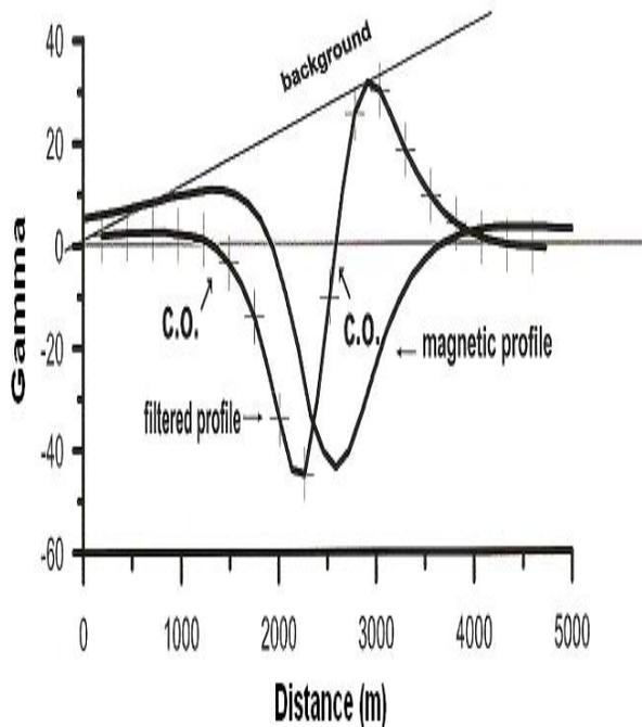
**Fig.(2a) Magnetic anomaly profile for dyke-like body (depth 500, width 500, inclination angle 10°) with its filtered profile using Fraser filter.**
