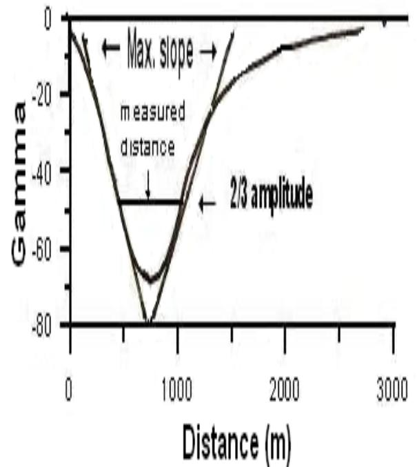
Fig.(5b) Residual curve obtained by subtracting Fraser filter values from background profile for the above magnetic profile.
