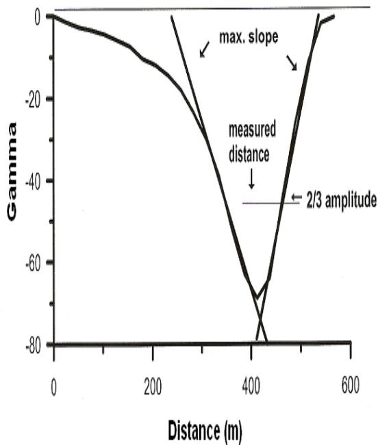
**Fig.(2b) Residual curve obtained by subtracting Fraser filter values from background for the above magnetic profile.**
