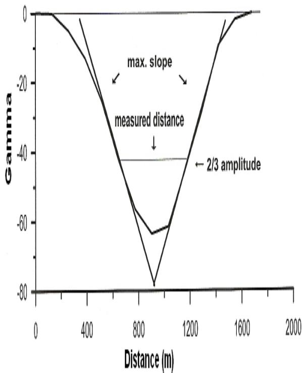
Fig.(3b) Residual curve obtained by subtracting Fraser filter values from background for the above magnetic profile.
