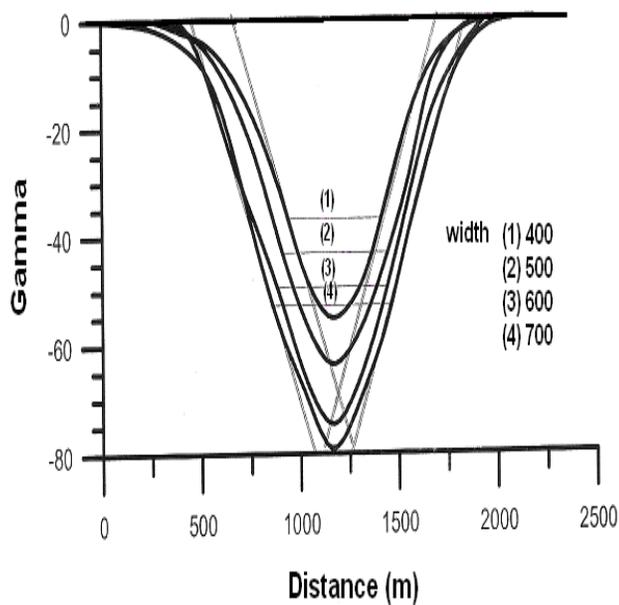
**Fig.(6)** Residual curve obtained by subtraction Fraser filter values from background for magnetic profile for dyke-like body with same depth of 500m, various widths and with inclination angle 40o.
