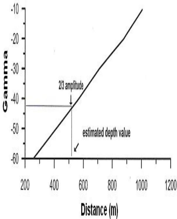
Fig.(4c) Depth estimation of dyke-like body from the relation of various amplitudes against distances between two straight lines of filtered profile.
