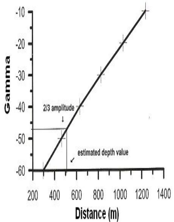
**Fig.(2c) Depth estimation of dyke-like body from the relation of various amplitudes against distances between two straight lines of filtered profile.**
