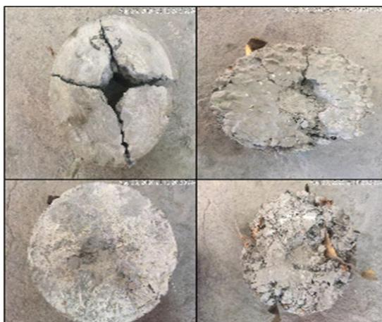
**Figure 9:** Failure of disc specimens under impact load
