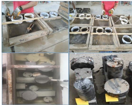
**Figure 3:** Stages of specimens' preparation
