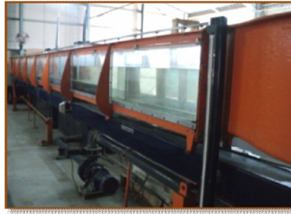
Figure (1): Hydraulic flume used in the present work
