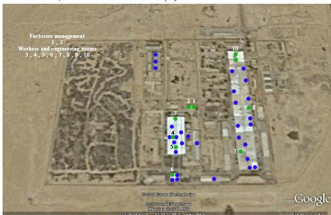
Figure (3): shows the sites of measured noise levels in the workers comfort places and in the factories management building.
