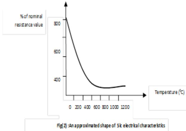
Fig(2):An approximated shape of Sic electrical characteristics
