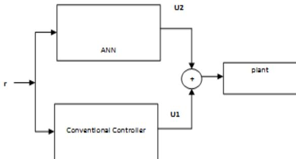
Figure (13) parallel neuro-control scheme
