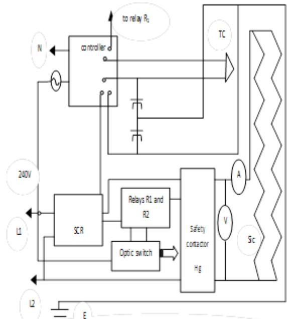
**Figure(6)Schematic diagram of SCR EF power control**
