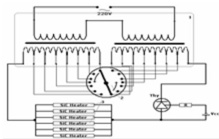
**Figure.(4)Power control using transformer**
