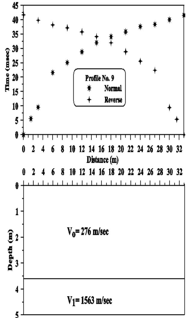
Fig. (4) The travel time curve for the profile No. (9) in the study area.
