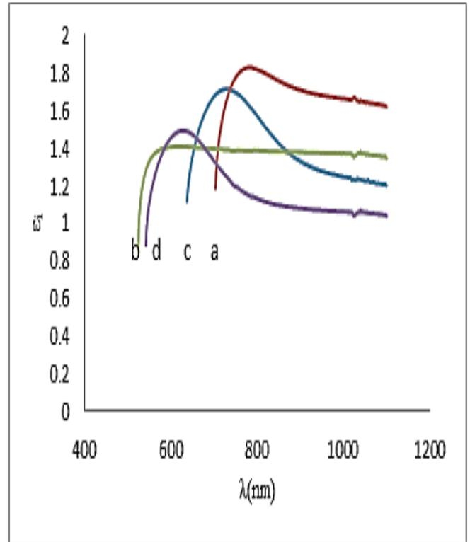
Fig.(7) The variation of imaginary dielectric constant with wavelength ( $\lambda$ ) for thin films prepared (a) CdIn<sub>2</sub>S<sub>4</sub>, (b) CdIn<sub>2</sub>S<sub>4</sub>:1%Cu, (c)CdIn<sub>2</sub>S<sub>4</sub>:3%Cu,(d) CdIn<sub>2</sub>S<sub>4</sub>:5%Cu
