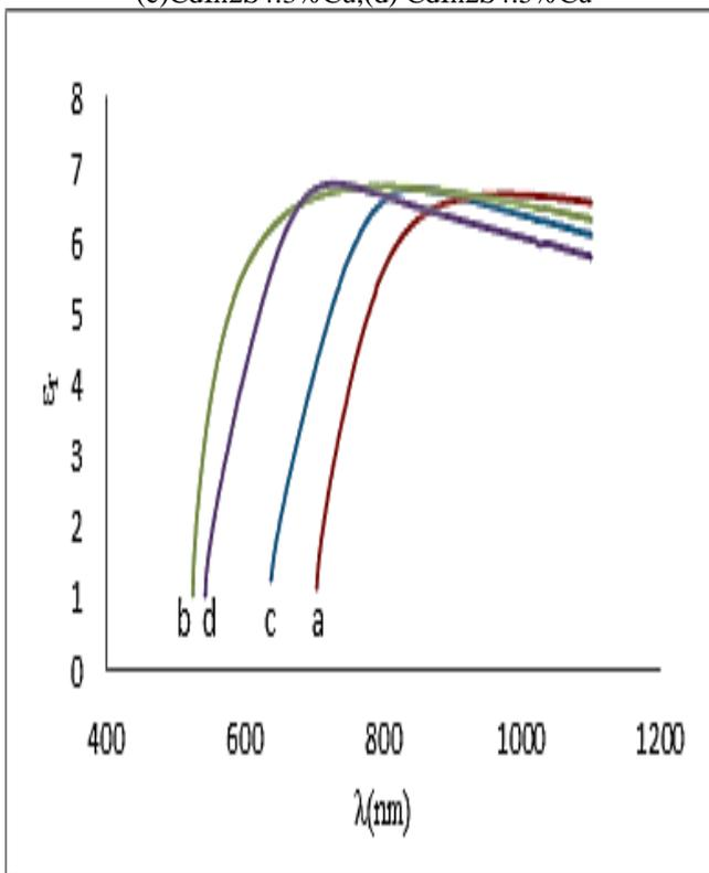
Fig.(6) The variation of real dielectric constant with wavelength ( $\lambda$ ) for thin films prepared (a) CdIn<sub>2</sub>S<sub>4</sub>, (b) CdIn<sub>2</sub>S<sub>4</sub>:1%Cu, (c)CdIn<sub>2</sub>S<sub>4</sub>:3%Cu,(d) CdIn<sub>2</sub>S<sub>4</sub>:5%Cu
