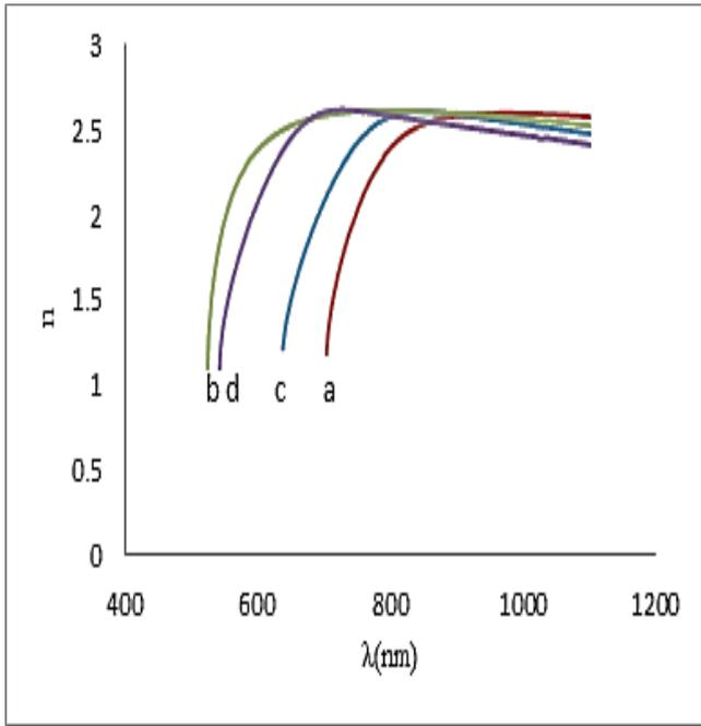
Fig.(5) The variation of refractive index (n) with wavelength ( $\lambda$ ) for thin films prepared (a) CdIn<sub>2</sub>S<sub>4</sub>, (b) CdIn<sub>2</sub>S<sub>4</sub>:1%Cu, (c)CdIn<sub>2</sub>S<sub>4</sub>:3%Cu,(d) CdIn<sub>2</sub>S<sub>4</sub>:5%Cu
