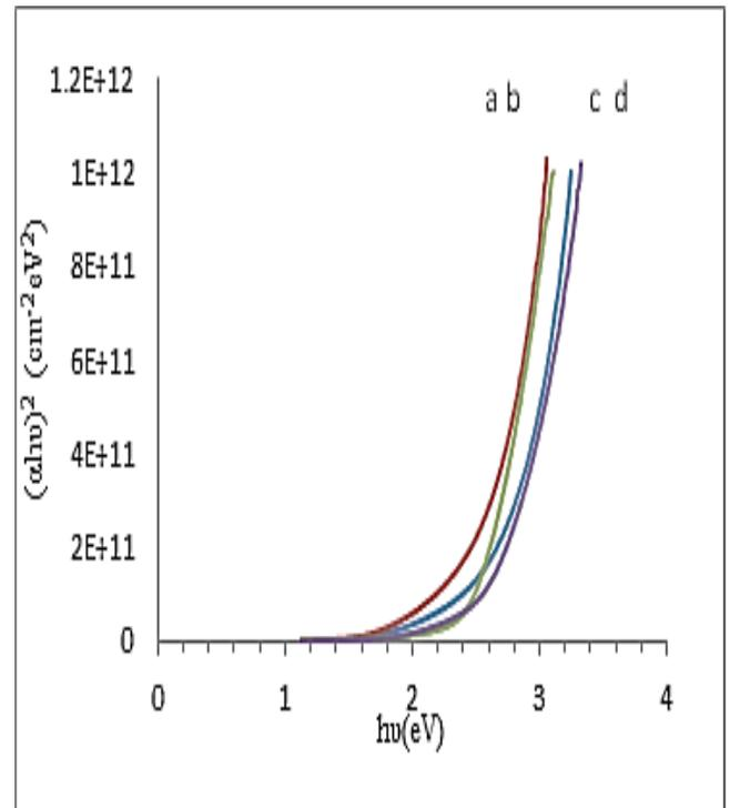
Fig (3) the optical energy gap ( $E_g$ ) value for thin films prepared (a) CdIn<sub>2</sub>S<sub>4</sub>, (b) CdIn<sub>2</sub>S<sub>4</sub>:1%Cu, (c)CdIn<sub>2</sub>S<sub>4</sub>:3%Cu,(d) CdIn<sub>2</sub>S<sub>4</sub>:5%Cu
