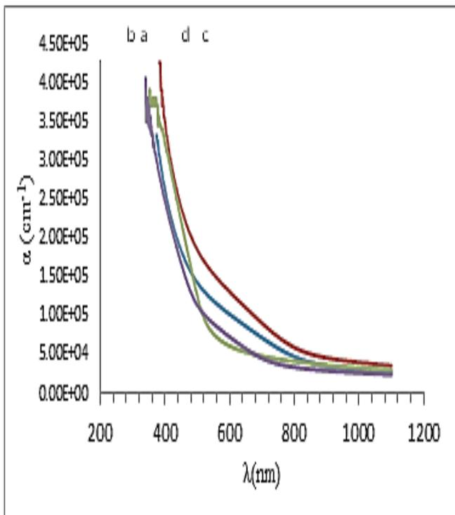
Fig.(2) the variation of absorbtion coefficient ( $\alpha$ )with wavelength ( $\lambda$ ) for thin films prepared (a) CdIn<sub>2</sub>S<sub>4</sub>, (b) CdIn<sub>2</sub>S<sub>4</sub>:1%Cu,(c) CdIn<sub>2</sub>S<sub>4</sub>:3%Cu, (d)CdIn<sub>2</sub>S<sub>4</sub>:5%Cu
