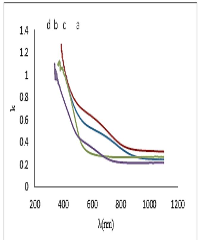
Fig.(4) The variation of extenction coefficient ( $k$ ) with wavelength ( $\lambda$ ) for thin films prepared (a) CdIn<sub>2</sub>S<sub>4</sub>, (b) CdIn<sub>2</sub>S<sub>4</sub>:1%Cu, (c)CdIn<sub>2</sub>S<sub>4</sub>:3%Cu,(d) CdIn<sub>2</sub>S<sub>4</sub>:5%Cu
