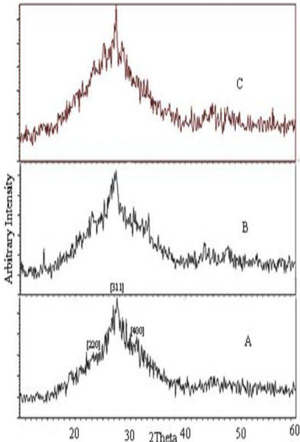
Fig. (1) The XRD pattern of CdIn<sub>2</sub>S<sub>4</sub> thin films(A)without doping, (B)doping 1%Cu,(C)doping 3%Cu
