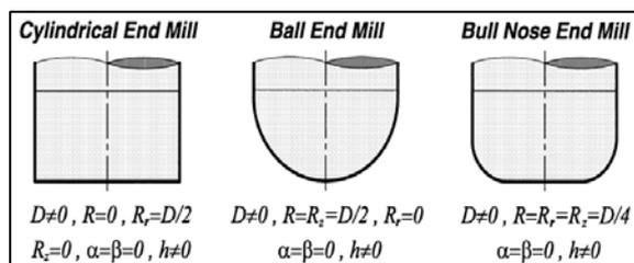
Figure 3: The end mill geometric parameters for the flat, ball and toroidal (bullnose) [10].
