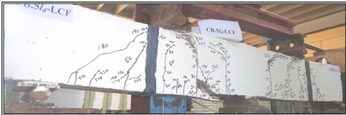
Fig. 14- Failure Mode of Girder CB.5I d -LCF
