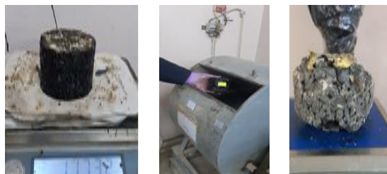
Figure (8): Specimen before and after Loss test
