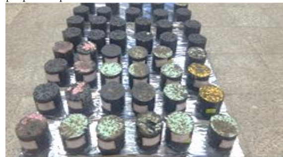
Figure (2): Some of the Prepared Marshall Specimens
