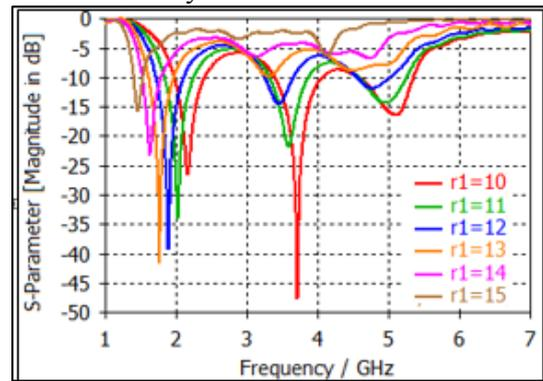
Figure 4: The simulated input reflection coefficients of the modeled antenna with  $R_1$  (mm) as a parameter
