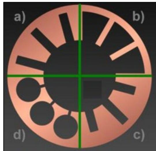
**Figure 1: The different forms of the resonant cavities constituting the anode block in a magnetron [13]**
