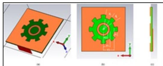
**Figure 2: The layout of the modeled antenna; (a) A perspective view, (b) A top view, and (c) A side view**
