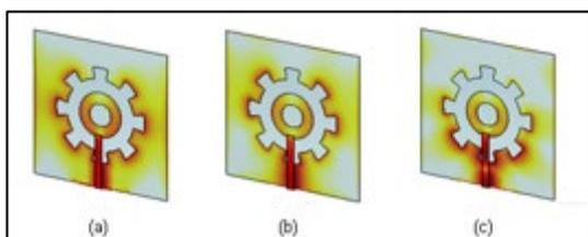
**Figure 9. The simulated current distributions on the surface of the proposed antenna at; (a) 2.4 GHz, (b) 3.5 GHz, and (c) 5.2 GHz**
