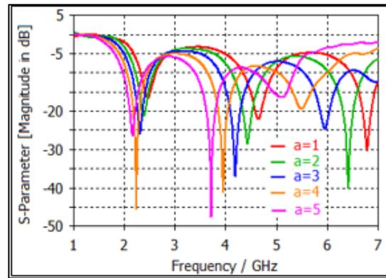
**Figure 3: The simulated input reflection coefficients of the modeled antenna with  $A$  (mm) as a parameter**
