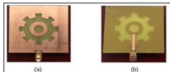
Figure 6: Photos of the fabricated prototype; (a) front view, and (b) the bottom view
