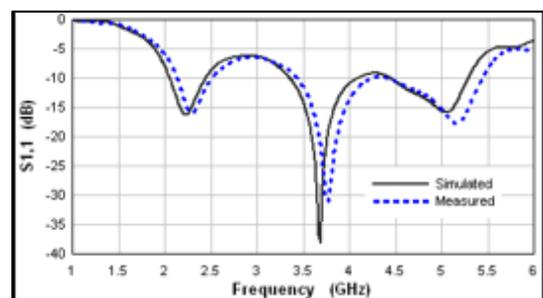
Figure 7: The simulated and measured input reflection coefficient responses of the fabricated antenna
