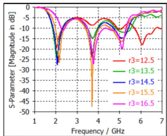
Figure 5: The simulated input reflection coefficient of the modeled antenna with  $R_3$  (mm) as a parameter
